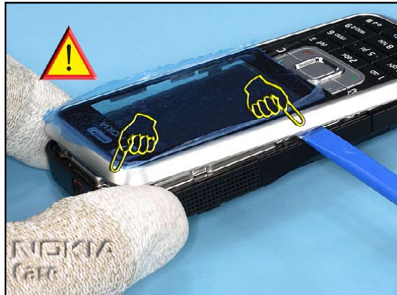
8. Then unlock the clips on the other side and remove the A-COVER.
