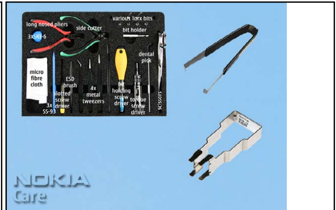
2. You will need the Nokia Standard Toolkit version 2 as well as the connector opening tool SS-34 and the camera removal tool SS-102. Also refer the General Mechanical Guideline Video for additional hints about the tools and component handling.
