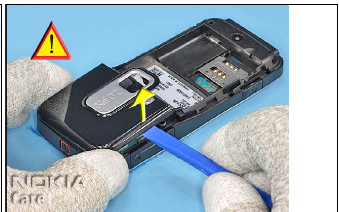
6. Release the last clip and remove the ANTENNA COVER ASSY.
