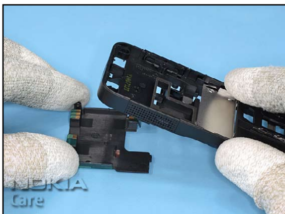
29. Now, the ANTENNA ASSY can be removed easily.
