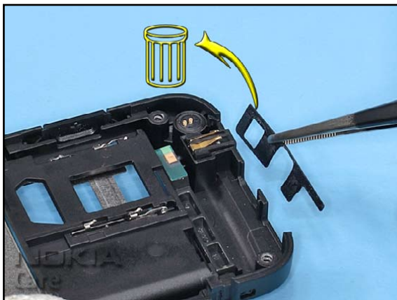
24. Remove the CONNECTOR LABEL and discard it.
