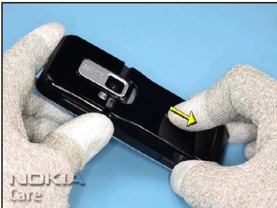
3. COVER all sensitive surfaces with a protective film. Unlock and remove the BATTERY COVER. Remove the Battery if inserted.
