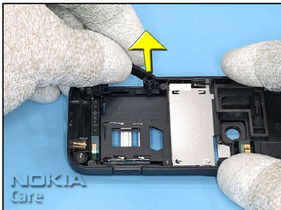
23. Open the MEMORY CARD DOOR and remove it.
