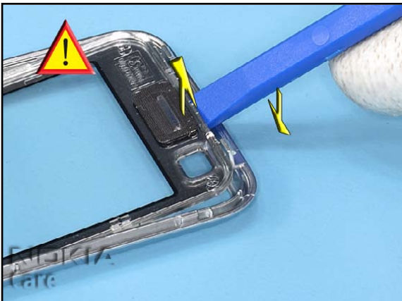
9. Unlock the WINDOW ASSY on the top of the COVER first.
