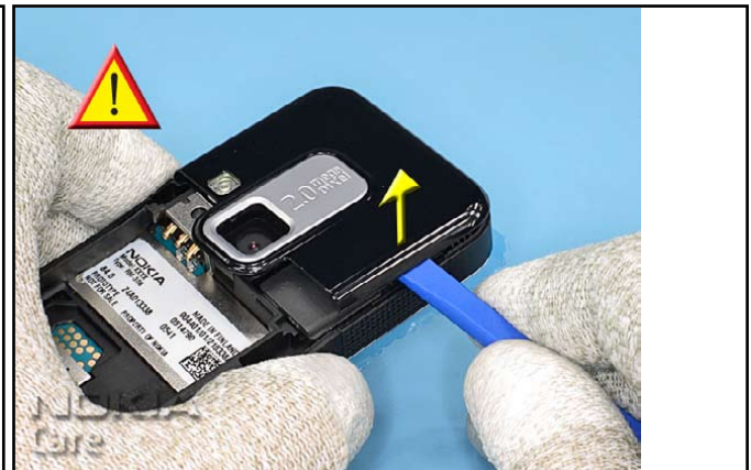
4. Place the SS-93 between the C-COVER and the ANTENNA COVER ASSY, and release the clips beginning on the shown side.
