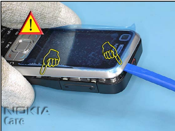
7. The A-COVER is attached with clips to the C-COVER. Unlock the clips on the shown side first. Avoid damaging the clips.
