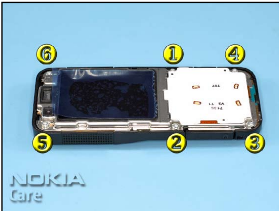
13. Undo the SCREWS in the order shown and remove them.
