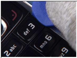
5. Carefully pry open the KEYMAT with SRT-6 at key 3.
