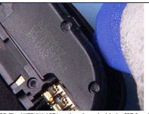
25. The ANTENNA ASSY can be released with the SRT-6 easily.
