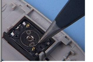
2. Ensure that the dust net is glued on the Earpiece, then place the EARPIECE evenly into the Gasket.
