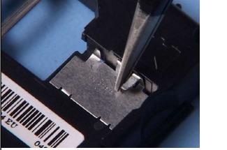
26. Use the tweezers to unlock the BATTERY SPRING.
