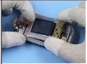
4. Put the NAPA DISPLAY Main into the B-COVER guides.
