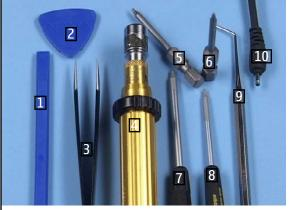
1. Needed tools: 1. SS-93, 2. SRT-6, Metal tweezers, 4. Torque driver, 5. Torx plus size 5 bit, 6. Torx plus size 6 bit, 7. Torx plus driver size 6, 8. Torx plus driver size 5, 9. Dental pick and 10. DC-Plug.
