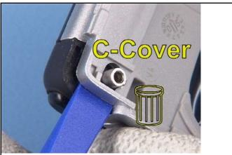
14. Loosen the C-COVER from the HINGE, also using the SS-93.
