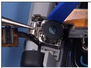
3. Position the Camera Assembly into the guides of the B-COVER. Take care not to damage the board to board or camera flex foil.
