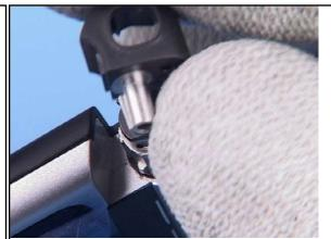
16. Remove the HINGE CAP RIGHT and then the Push to Open Button.
