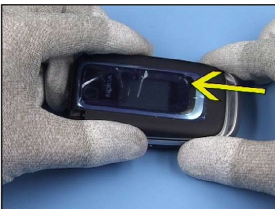
12. You can now remove the A-Cover by sliding it and lifting it off as shown.
