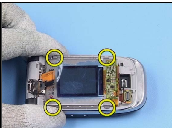
18. Unlock the four clips with holding the NAPA DISPLAY MAIN.
