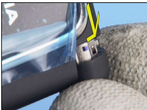
15. Only one position is possible for the HINGE CAP RIGHT assembly.
