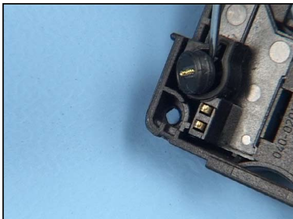
19. Ease out the Microphone with the dental pick.
