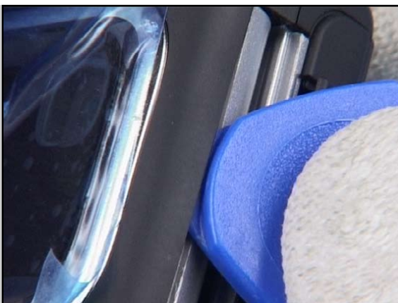
10. Now, run the SRT-6 along the joint as shown to release the concealed snaps.
