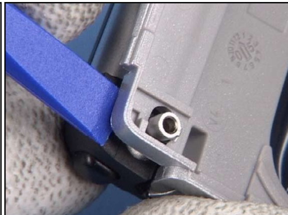
10. Use the SS-93 to release the C-COVER from the Hinge.
