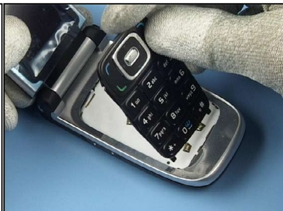
24. Finally, assemble the KEYMAT, starting from the lower side.
