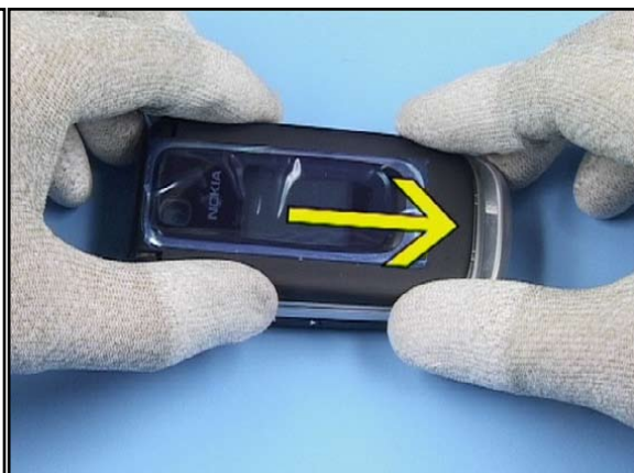
12. Slide the A-Cover on to its lower guides.
