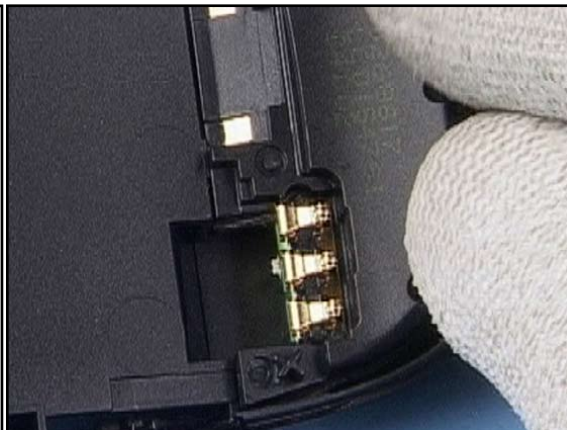
2. Insert the ANTENNA MODULE into its compartment.
