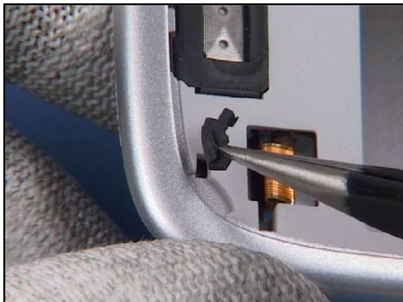
7. Remove both RUBBER STOPPERS with tweezers.
