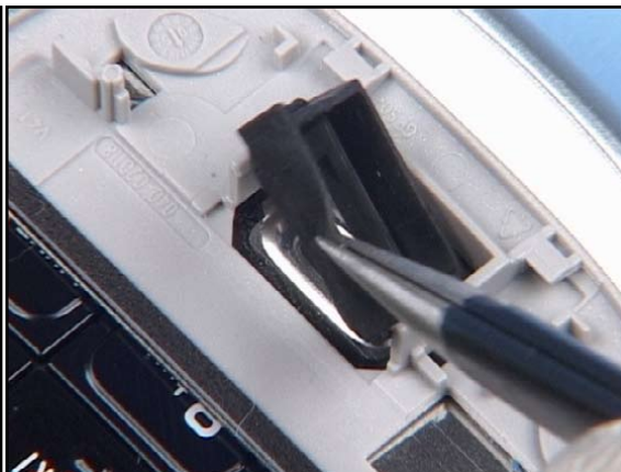
20. Remove the EARPIECE GASKET with tweezers.
