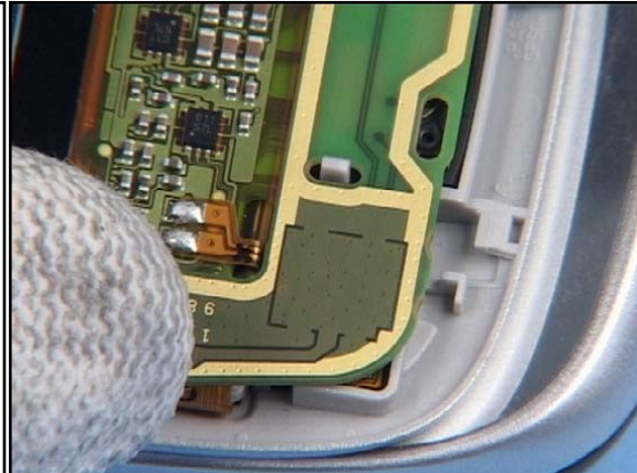
8. Ensure that the LCD connector is properly locked.
