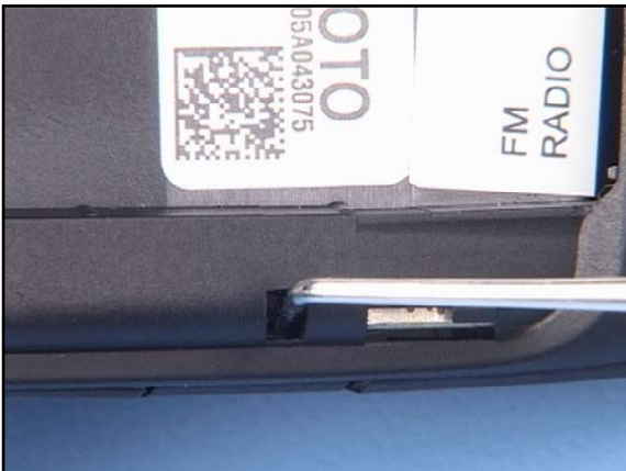
9. Use the dental pick to unlock the clips at both sides.
