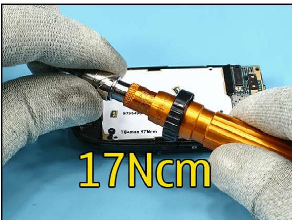
11. Set the correct torque and tighten in.
