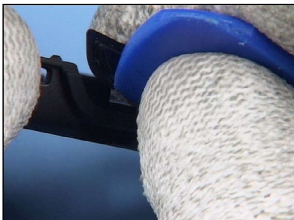
17. Release all buttons with the SRT-6 as shown.
