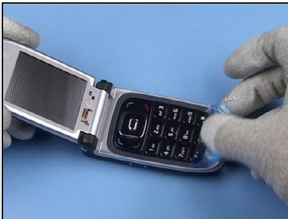
8. Protect the inner side of the lower block with film.
