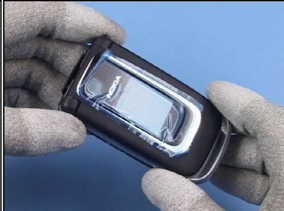
2. Always protect all windows with protective film against dust and scratches.
