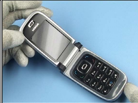
26. Check all windows for cleanliness.
