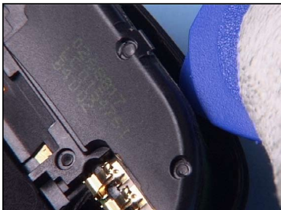
21. The Antenna Assembly can be released easily with the SRT-6.
