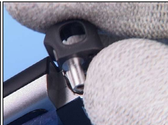
12. Remove the HINGE CAP RIGHT and then the Push to Open Button.
