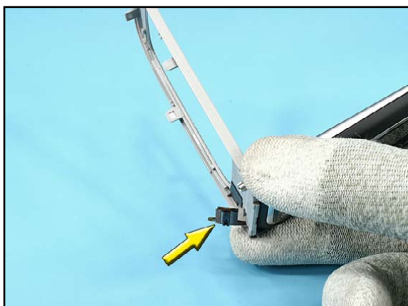
17. Position the C-COVER SERVICE ASSY in 90 degrees angle to the Upper BLOCK.
