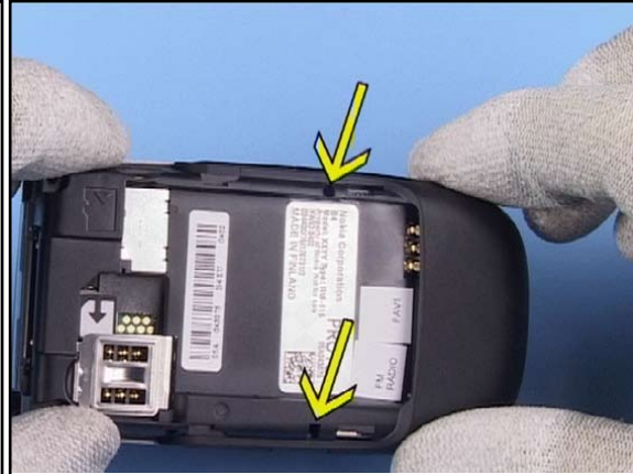
8. Hold the assembly as shown and locate the 2 holes in the D-COVER.
