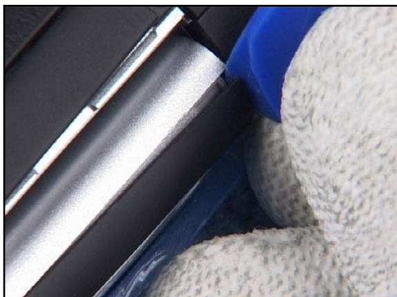
9. Gently unlock the A-COVER at the back.
