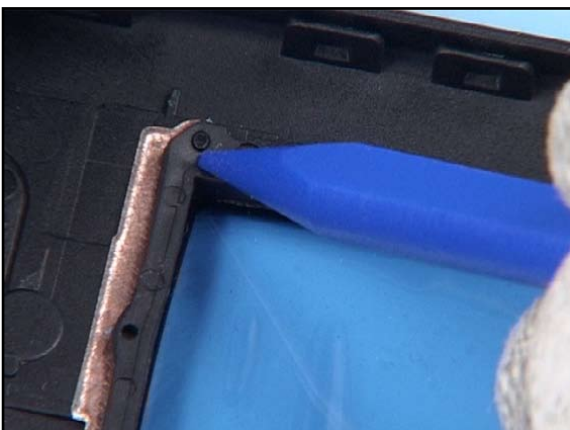
11. Put the FRONT DISPLAY GASKET to the A-COVER.
