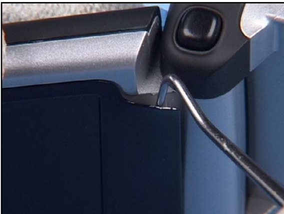
5. Carefully lift up the lower side of the DISPLAY BEZEL with the dental pick...
