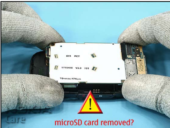
9. Place the ENGINE BOARD into the D-COVER.
