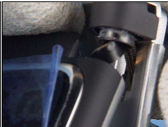
14. Be sure not to squash the FLEX FOIL when assembling the HINGE.
