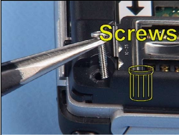
7. These screws are coated with locking compound and cannot be reused.
