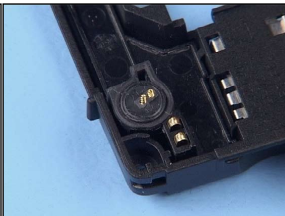
4. Carefully insert the MICROPHONE into its compartment.
