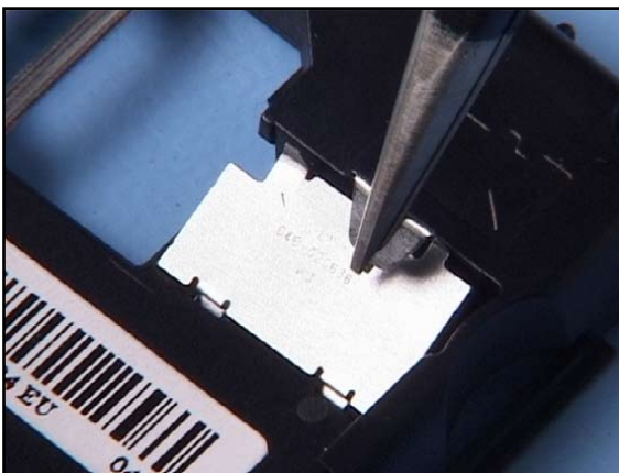
22. Use the tweezers to unlock the BATTERY SPRING.
