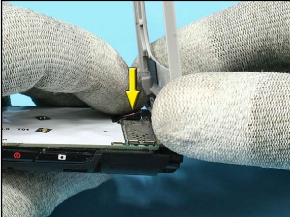
19. Press onto the flex connector. A “click” noise can be heard when the connector lock properly.
