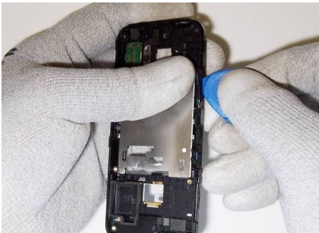
15) Use SRT-6 to get under volume key. Lift up the volume key and remove it.
