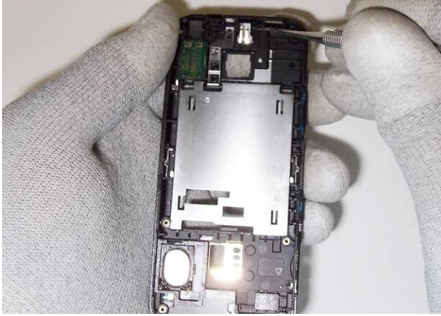
13) Use dental tool to lift DC jack.
