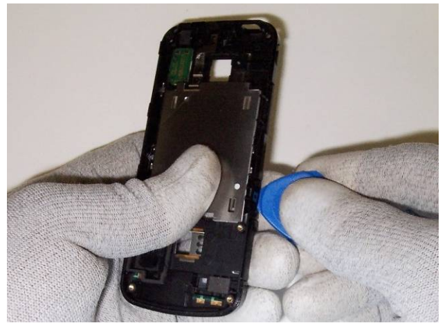
16) Use SRT-6 to get under camera key. Lift up the camera key and remove it.
