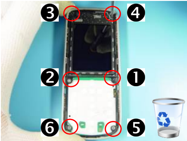
13) Unscrew the six T6+ screws in the order shown and discard them.
