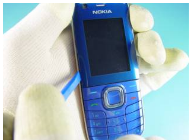
6) Open the first clip on the other side of the DISPLAY WINDOW ASSY.
