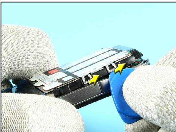
17. Unlock the four clips of the C-COVER PLATE ASSY and loosen it.
