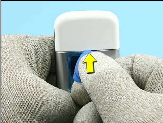
13. Stick the SRT-6 into between the TOP COVER and the CAMERA BEZEL and release the TOP COVER.
