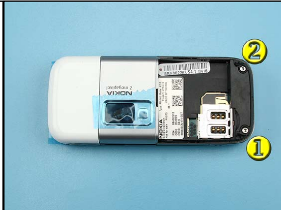
4. Undo the Torx Plus size 6 screws in the order shown. For assembly, use the reverse order and a torque of 27 Ncm.
