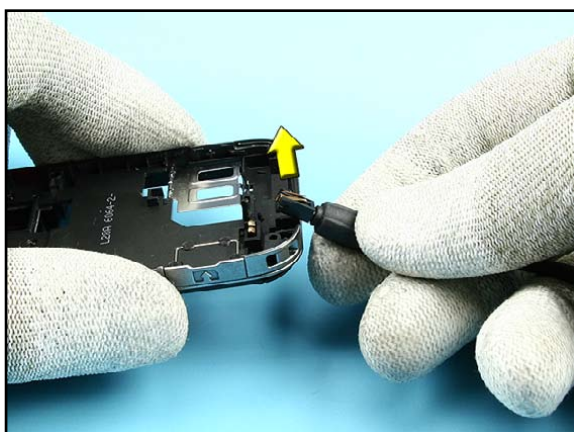
29. Remove the DC-JACK with a DC-plug.
