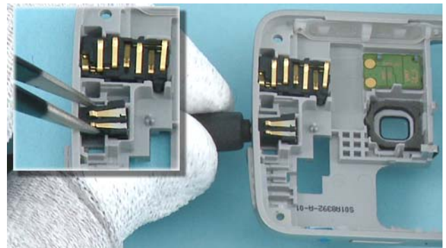
24) Release the AV JACK and the DC JACK with the DC plug and remove them with the tweezers.
