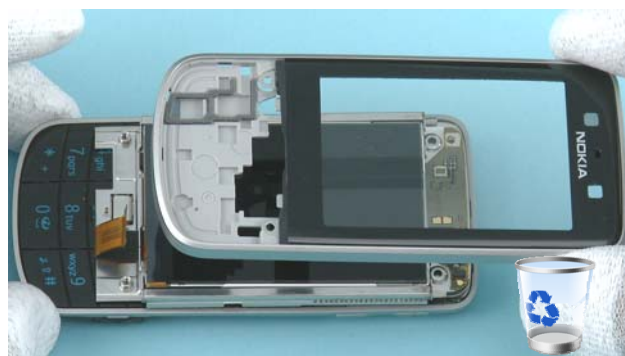
10) The A-COVER ASSY can now be removed. Remember to protect the LCD with protective film.
