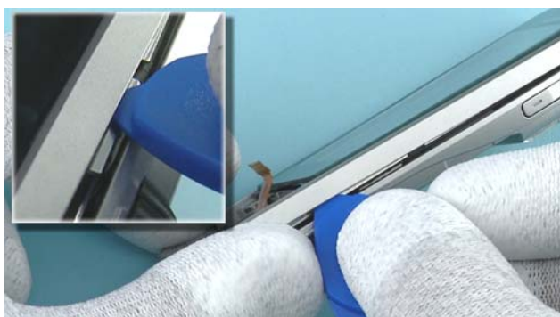
9) Use the SRT-6 to open the two clips of the A-COVER ASSY. Slide the SRT-6 along the cover edge. Do the same on the opposite side.
