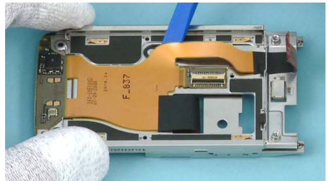
30) Carefully loosen up the adhesive on the MAIN FLEX with the SS-93 as shown.
