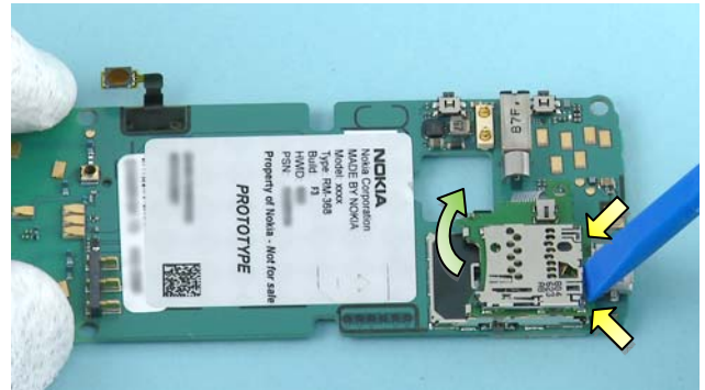
28) Release the two clips holding the MICRO SD PWB ASSEMBLY. Lift up the assembly to get access to the connector.
