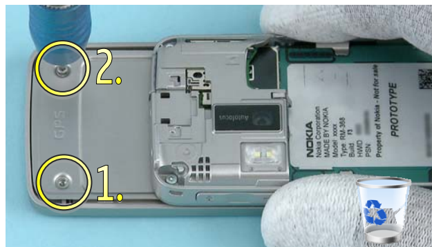
8) Turn the phone over and slide it open. Then unscrew these two Torx+ 4 screws in the order shown.
