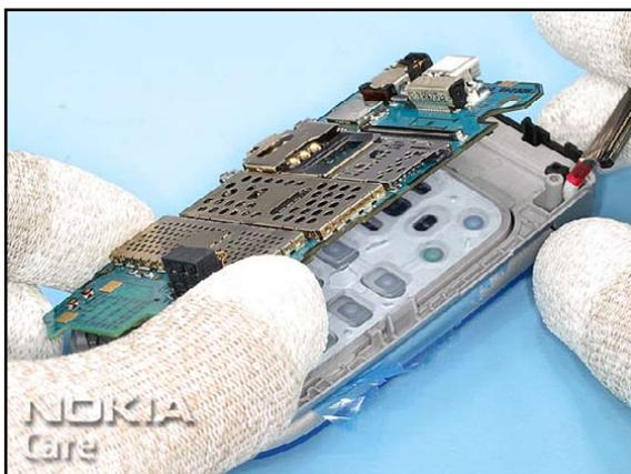
18. Now the ENGINE MODULE can be removed.
