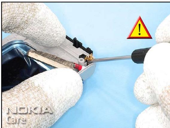
22. Ease out the HINGE GROUNDING CLIP carefully with a straight bladed screwdriver.. Do not scratch the coax cable underneath.
