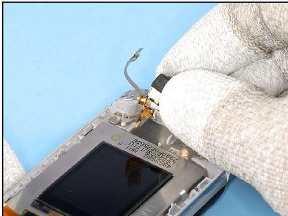
18. Lift out the 1ZC-D CAMERA FLEX. Mind the sharp metal latches on order to avoid cutting the delicate flex foil. It is not necessary to remove the camera flex if the CAMERA MODULE should be replaced only. In this case simply peel up the CAMERA GASKET and lift out the CAMERA MODULE with the SS-45.
