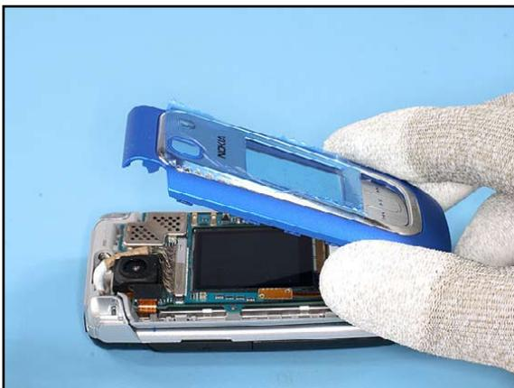
10. Now lift up the A-COVER ASSY, beginning from the hinge side in order to release the last 2 clips.
