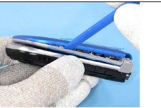
8. Carefully pry open the 5 clips of the A-COVER ASSY...
