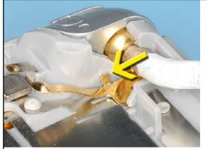
1. Assembly hints: Mind the correct positioning of the COAX ASSEMBLY before going on. Note that the grounding clip is positioned correctly. It must be clicked into its place as shown.
