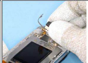
18. Lift out the 1ZC-D CAMERA FLEX. Mind the sharp metal latches on order to avoid cutting the delicate flex foil. It is not necessary to remove the camera flex if the CAMERA MODULE should be replaced only. In this case simply peel up the CAMERA GASKET and lift out the CAMERA MODULE with the SS-45.
