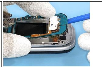
14. Carefully lever up the TOP BOARD MECH ASSY. Keep in mind that a flex foil is still connected.
