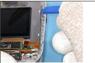
20. Unlock the plastic clips of the LCD MODULE.
