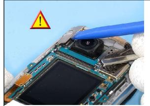
13. Carefully open the flex connector with the SS-93. Avoid mechanical stress to the connector and the flex foil.
