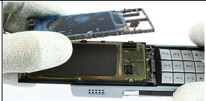
20. Remove the LCD Frame Assy.
