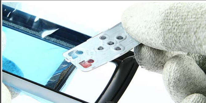
13. Protect the inner side of the window with a plastic film and separate the Function Keymat.
