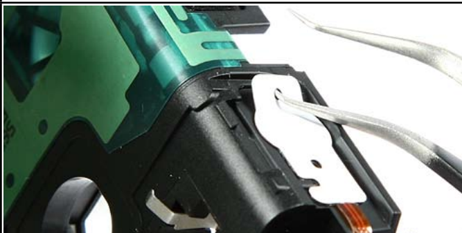
37. Peel up the Side Key Flex Assy with angled tweezers at the shown side first.
