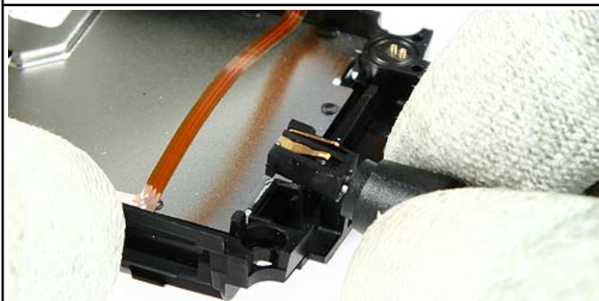
31. Remove the DC-Jack with the DC plug.
