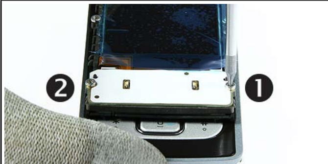
15. Remove 2 Torx Plus® size 6 screws in the order shown. For assembly, use the reverse order and a torque of 14 Ncm.
