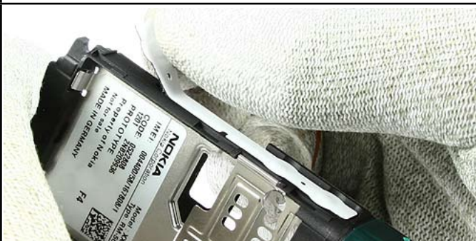
39. Continue with the larger part. Peel it up slowly to prevent adhesive residues.
