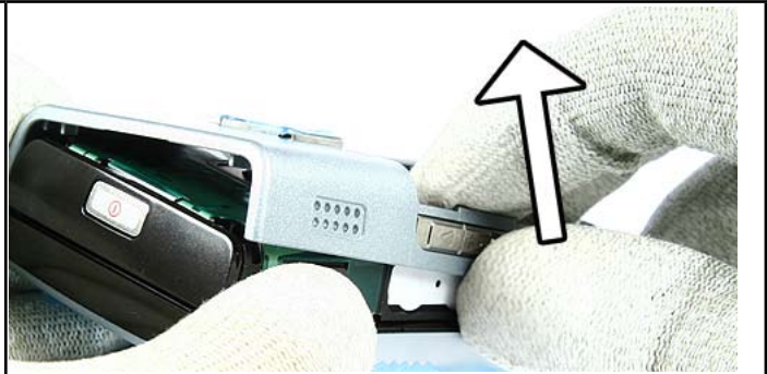
14. Carefully lift the Back Cover Assy from one side first. Place the connector side first when reassemble.
