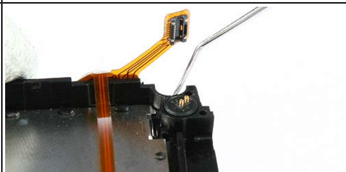
32. Remove the Microphone with the dental tool.
