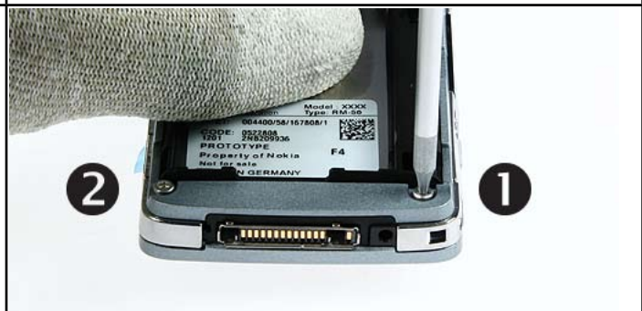
8. Remove the 2 Torx Plus® size 6 screws in the order shown. For assembly use the reverse order and a torque of 14 Ncm.
