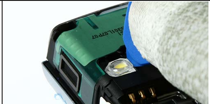
18. Release the Flash Light with the SRT-6.
