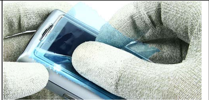
2. Protect the window with a plastic film.
