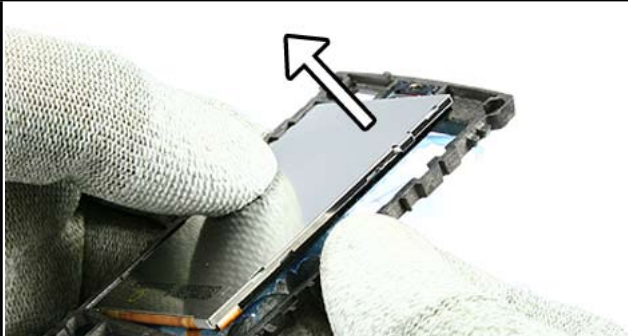
21. Separate the LCD from the Frame.
