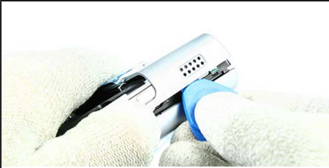
13. Release the clips of the Back Cover Assy on both sides as shown.
