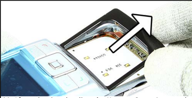
11. After releasing the clips, the Keymat Cover Assy can be removed easily.
