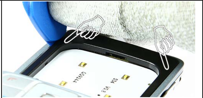
10. Release the plastic clips of the Keymat Cover Assy.
