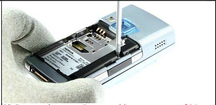
12. Remove the screw. For assembly use a torque of 14 Ncm.
