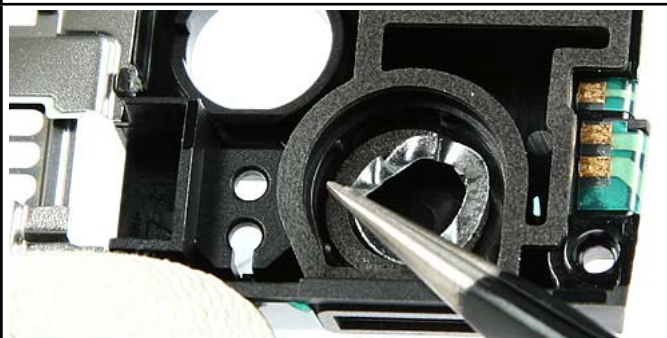
35. Peel up the Adhesive residues with tweezers. Always use new ones when reassemble.
