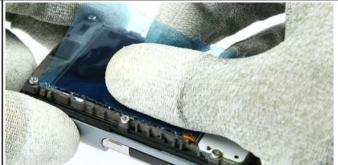
14. Protect the LCD with a plastic film, too.
