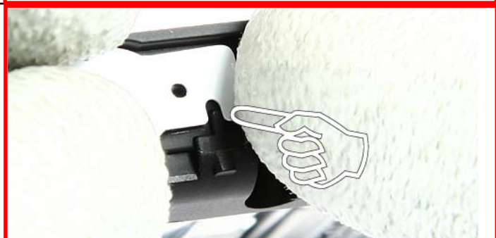
40. For Assembly mind the correct positioning of the Side Key Flex Assy.
