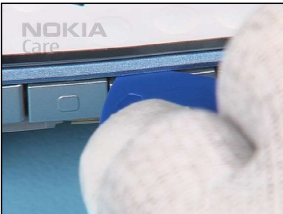
11. Place the SRT-6 between the C-COVER ASSY and the A-COVER LOWER and carefully release the snaps.
