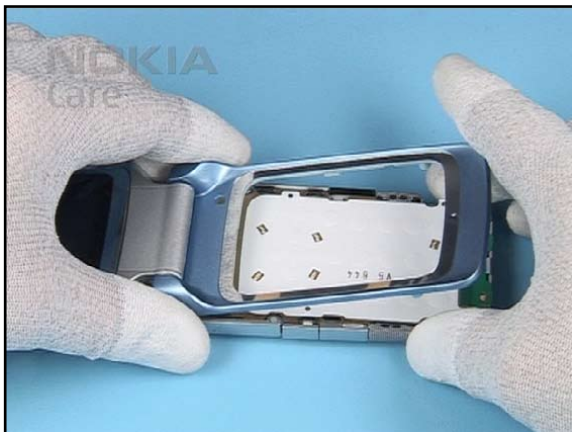
12. Lift the A-COVER LOWER as shown...
