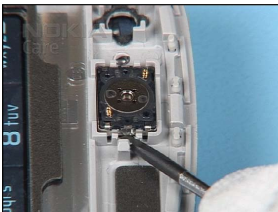
22. Use the flat bladed screwdriver as a lever to unlock the EARPIECE from its place...
