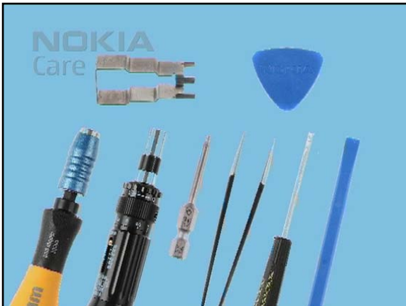
1. Needed tools : A Torx and a torque driver, a Torx Plus size 6 bit, metal tweezers, a flat bladed screwdriver, the SS-93, the SRT-6 and the SS-102 camera removal tool.
