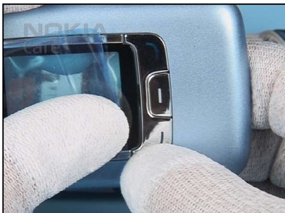
15. Fit the UI KEYMAT and close the snaps.
