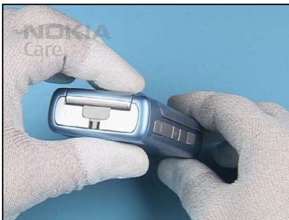
24. Finally, check that no gaps remain.
