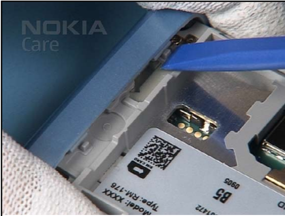
7. Unlock the snaps of the TOP CAP ASSY with the SS-93.
