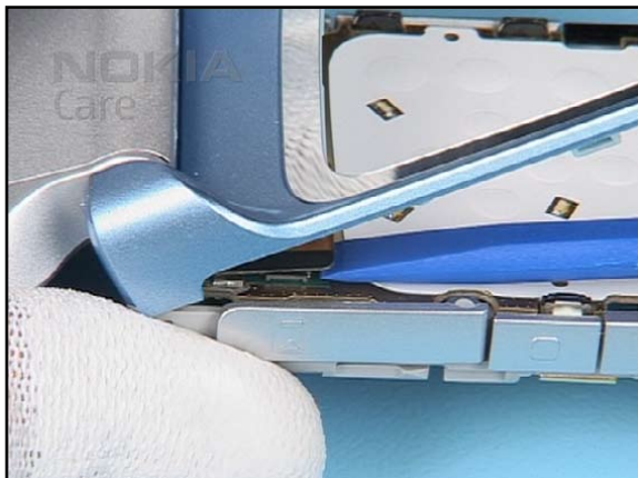
13. ...and carefully open the Hinge PWB FLEX connector with the SS-93.
