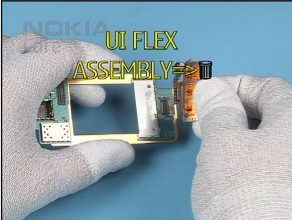
25. Remove the UI FLEX from the UI BOARD and discard it.
