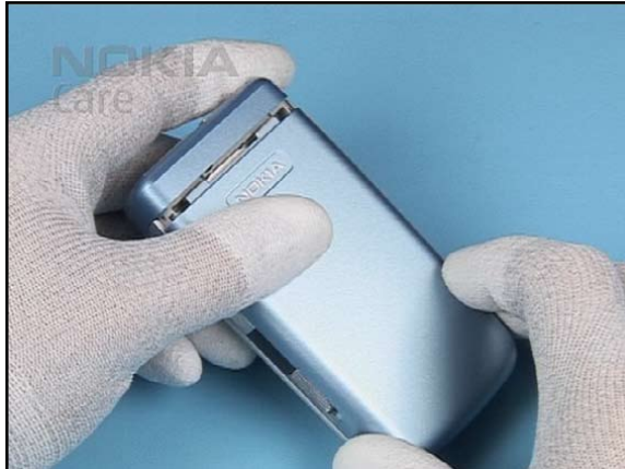
2. Open and remove the BATTERY COVER. Remove the Battery if inserted.
