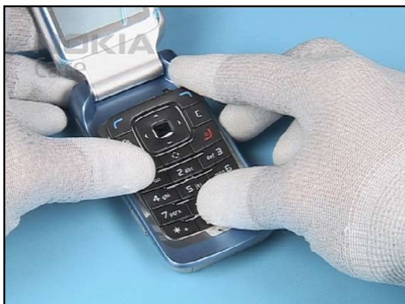
21. ...and fit the KEYMAT into the A-COVER LOWER.
