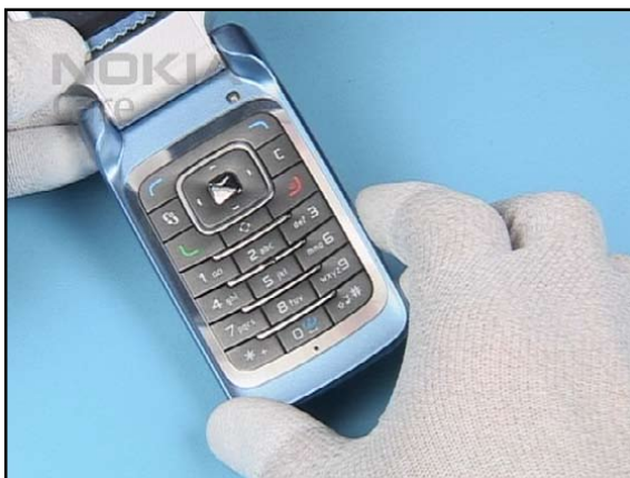
22. Check the correct position of the KEYMAT.
