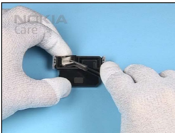
22. Now, remove the IHF SPEAKER. Do the same on the other side.
