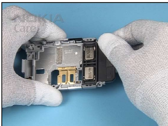
17. Remove the IHF ASSEMBLY from the C-COVER ASSEMBLY.
