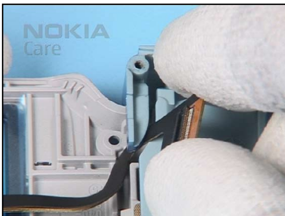
24. ...and remove the PWB FLEX from the HINGE.
