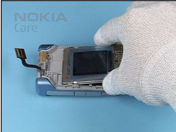
7. Place the LCD into the A-COVER UPPER.
