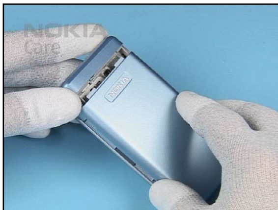
24. Finally, fit the BATTERY COVER.
