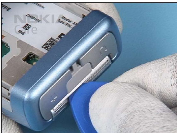
3. First, place the SRT-6 between the edge of the A-COVER UPPER and the A-COVER DECO PLATE and gently slide it along the edge.
