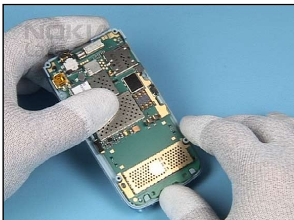
9. Note the right position of the guide pins.
