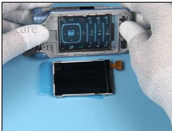
20. Now, the displays can be removed easily.
