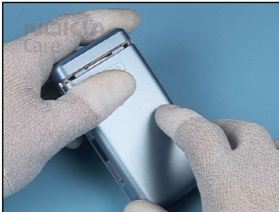
2. Open and remove the BATTERY COVER. Remove the battery if inserted.
