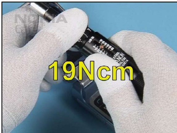
19. Set the torque driver to the correct torque.
