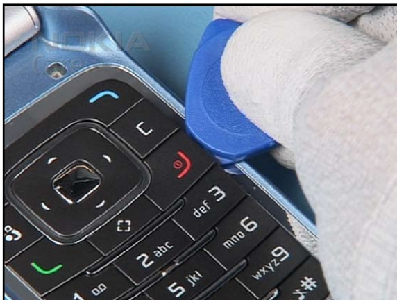
4. Place the SRT-6 between the KEYMAT and the A-COVER LOWER and carefully slide it along the edge as shown.
