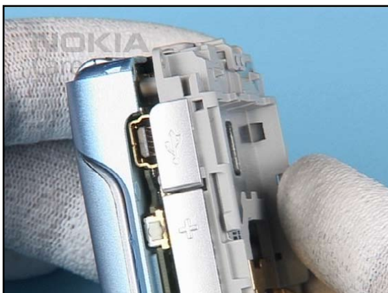
10. Align the C-COVER ASSY with the A-COVER LOWER.
