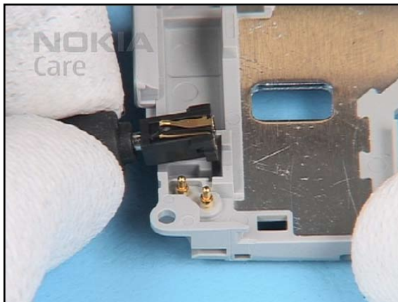
20. Use the DC-plug to remove the DC-JACK.
