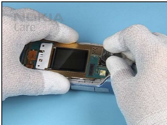
13. Secure the CAMERA MODULE by gently pressing it into place.
