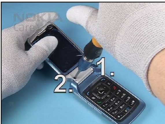
5. Unscrew the screws in the order shown.
