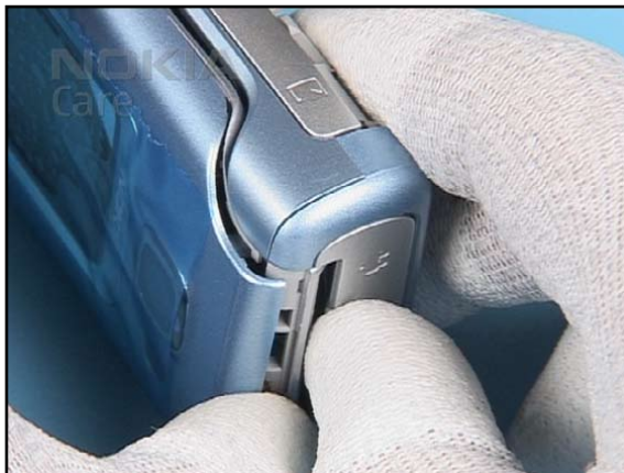
8. Expand the B-COVER UPPER from the shown side...
