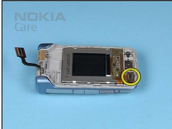
8. Ensure the right position of the LCD connector.
