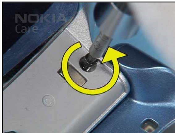
20. To avoid damaging of the plastic threads first tighten the screws to the left.
