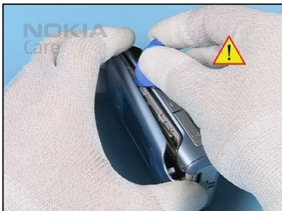
9. ...and gently slide the SRT-6 along the edge to unlock the snaps. Do not twist the SRT-6 to avoid scratching the covers.
