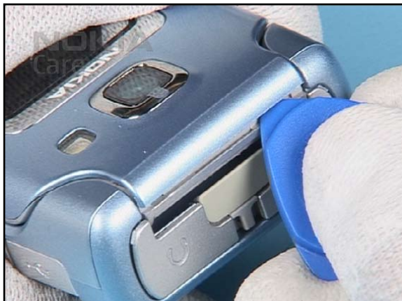
7. Unlock the snaps of the B-COVER UPPER starting on the shown side.
