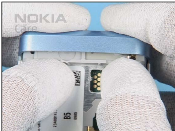
19. ...secure it by pressing it into position.
