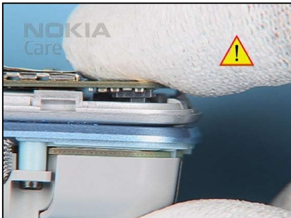
10. ...and carefully close the LCD connector.
