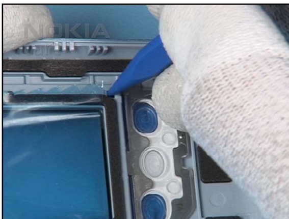
12. Unlock the snaps of the UI KEYMAT with the SS-93...
