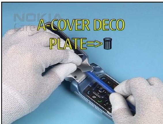
4. Then remove the A-COVER DECO PLATE with the SS-93 and discard it.
