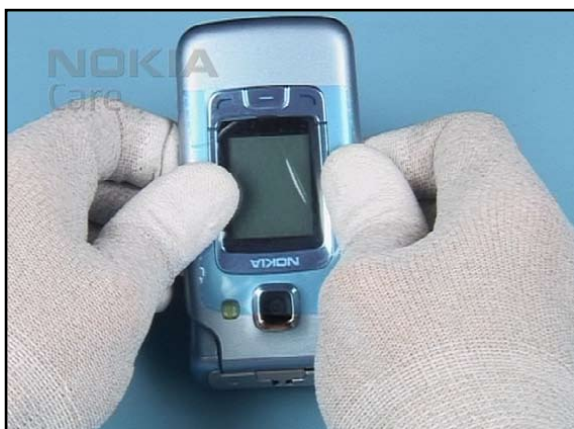
17. and carefully squeeze the parts together.
