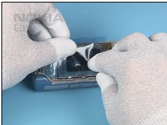
19. Cover the SUB DISPLAY with the protective film.
