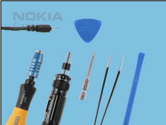
1. Needed tools: A Torx and a torque driver, a Torx Plus size 6 bit, metal tweezers, the SS-93, the SRT-6 and the DC-plug.
