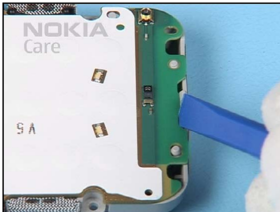
14. Unlock the ENGINE MODULE as shown...
