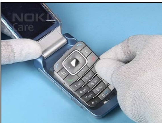
5. Remove the KEYMAT avoiding to touch the LEDs.
