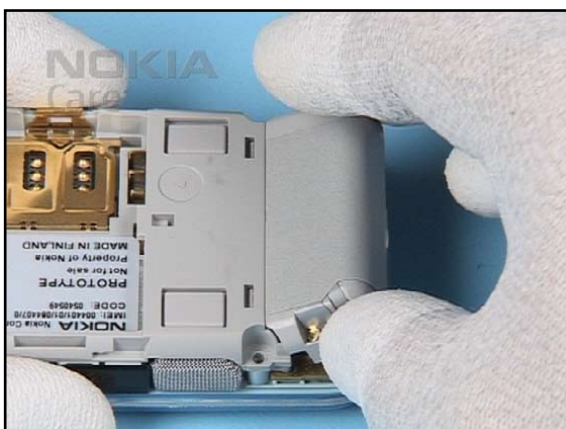
12. Fit the ANTENNA to the C-COVER ASSEMBLY...
