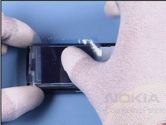
13. Cover the display with a film.
