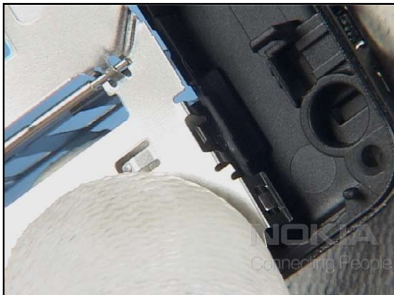
4. Carefully push all latches into their places.
