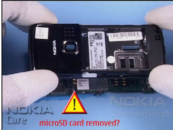
14. Note! Before removing the B-COVER, make sure that the micro SD card has been removed. Turn the assembly, lift up the B-COVER.
