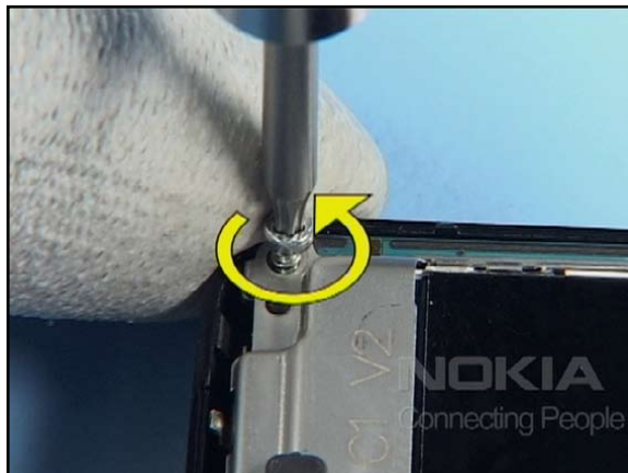
16. Turn the screws to the left first to engage the threads, then tighten them slightly.
