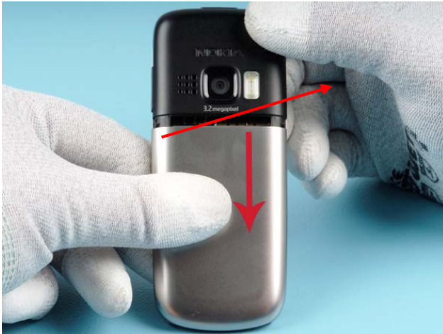
1) Open the C-COVER by sliding the cover as shown.
