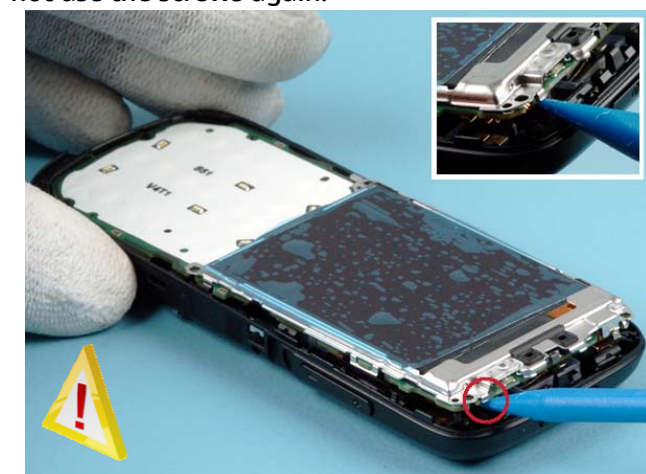
14) Use the SS-93 tool to release the clip on top to lift up the PWB incl. UI SHIELDING ASSY and LCD. Be careful not to damage the components on the PWB!
