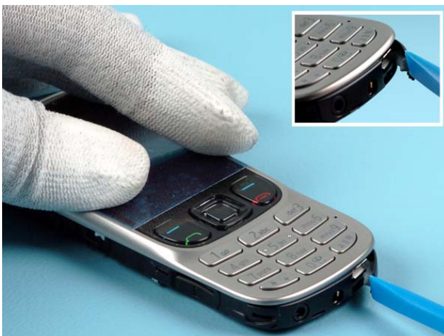
4) Use the SS-93 tool to open the USB COVER to have better access on the bottom side.
