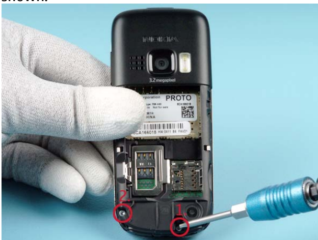
3a) Unscrew the two T6+ screws.
