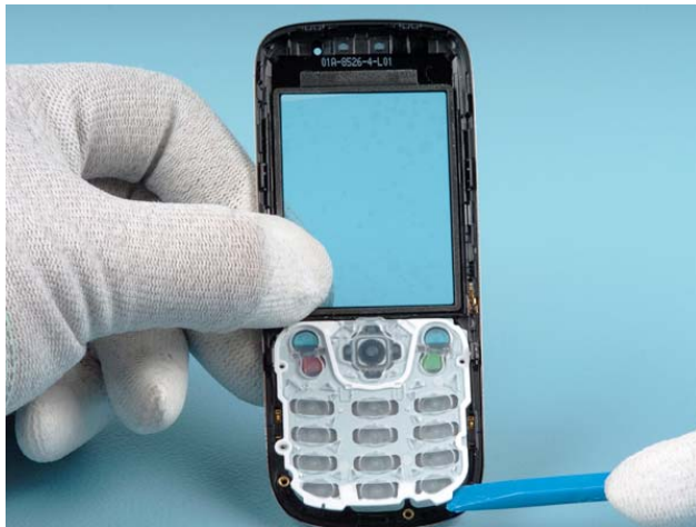
10) Use the SS-93 tool to release the KEYMAT ASSY.
