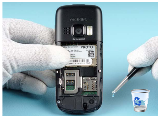
3b) Remove the screws with the tweezers. Do not use the screws again.
