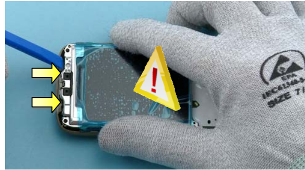
14) Use the SS-93 to detach the clips on top side of the device. Be careful not to damage the components on the engine board!
