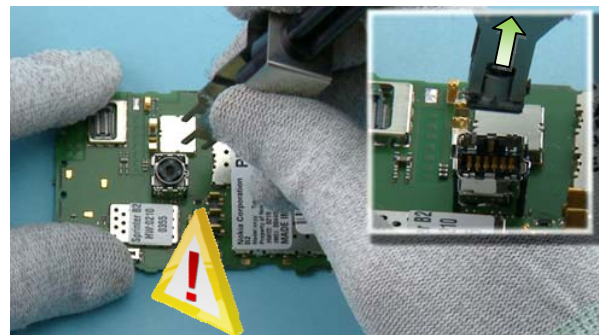
24) Push down the SS-88 camera removal tool to release the CAMERA retaining clips. Lift up the SS-88 and remove the CAMERA.
