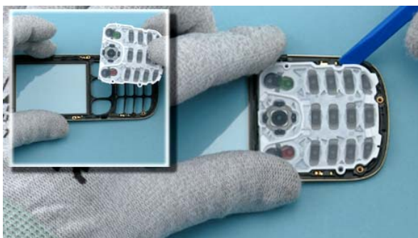
11) Use the SS-93 to separate the KEYMAT ASSY from the A-COVER. Remove the KEYMAT ASSY.
