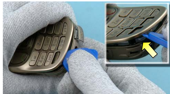
6) Insert the SRT-6 between the A-COVER and B-COVER to release the snaps of the A-COVER. First release the snap on the bottom side of the device.
