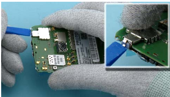
17) Open the clip of the FLEX SHIELDING with the SS-93.
