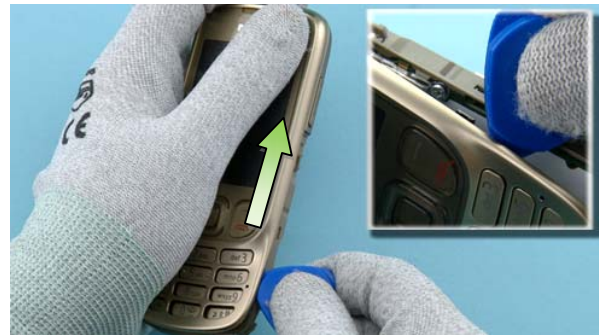
8) Then release the snaps along the edges on the other side of the device.
