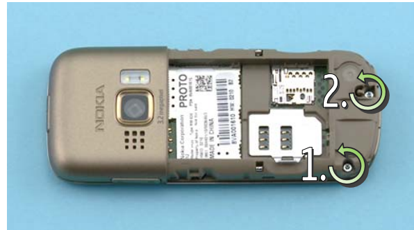
4) Unscrew the two TORX+ size 6 screws in the order shown. Discard them.
