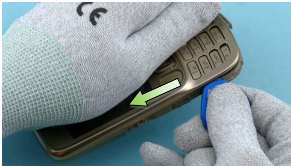
7) Slide the SRT-6 along the edges of the device to release the remaining snaps.
