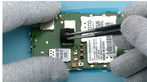
16) Use the tweezers to remove the CAMERA GASKET.
