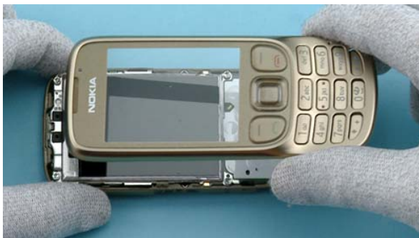
9) Remove the A-COVER and the KEYMAT ASSY.
