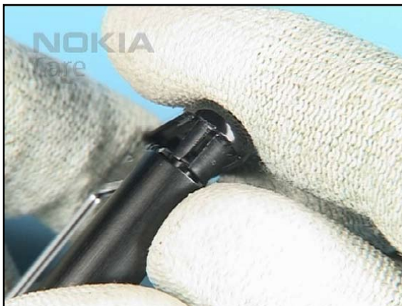
34. Always use a new TOP COVER ASSEMBLY. Pay attention to the correct position of the TOP COVER...
