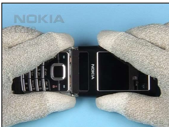
9. Carefully pull out the A-COVER.
