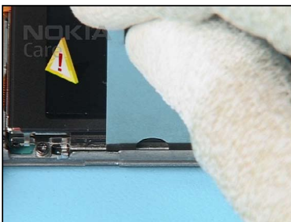
12. Place the SS-42 between the LCD FRAME and the C-COVER. Gently lever out the LCD FRAME.
