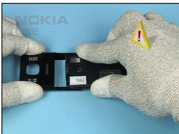
29. Align the A-COVER with the C-COVER. Do not slide the parts together yet.
