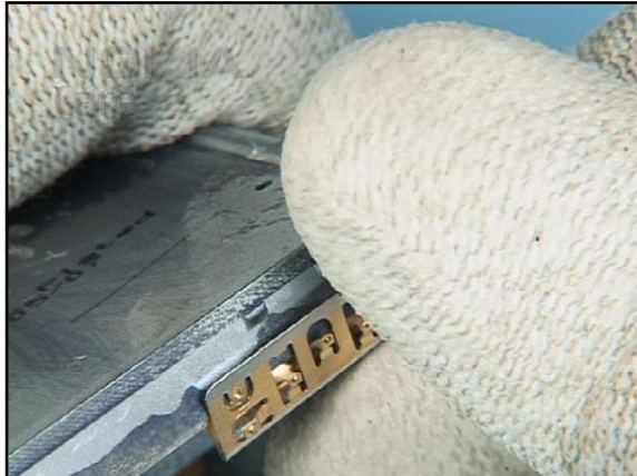
38. Unlock and remove the ANTENNA GROUNDING. The disassembly procedure is now finished.
