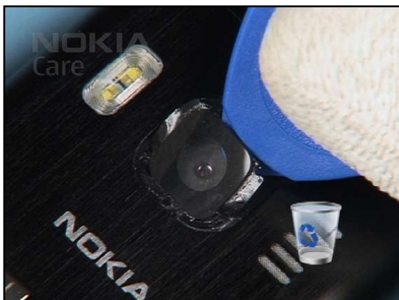
7. Then remove the window with the SRT-6 and discard it, too.
