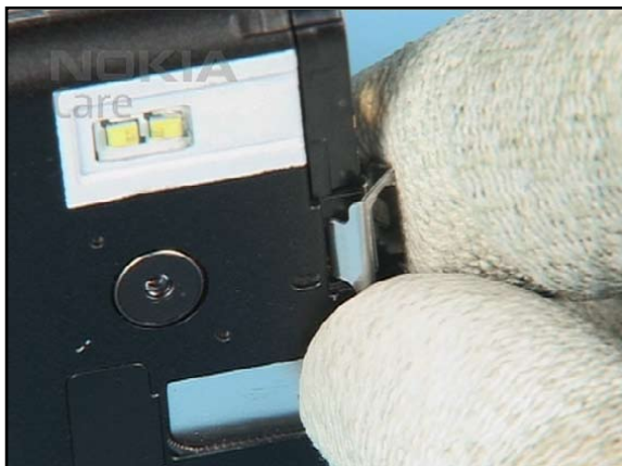
17. Fit the USB BRACE into the C-COVER at the shown side first...
