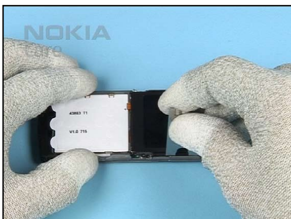
11. Release the LCD FRAME with the SS-42.
