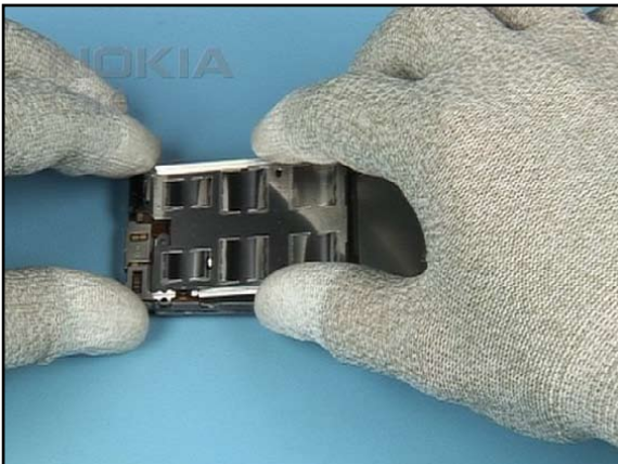
21. Align the DISPLAY BACK PLATE with the C-COVER.
