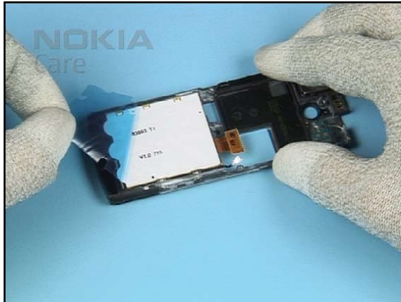
8. Remove the protection film from the UI FLEX.
