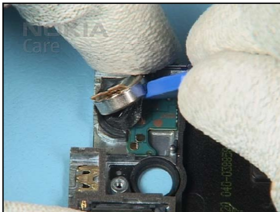
32. Remove the VIBRA and ensure that no adhesive remains.
