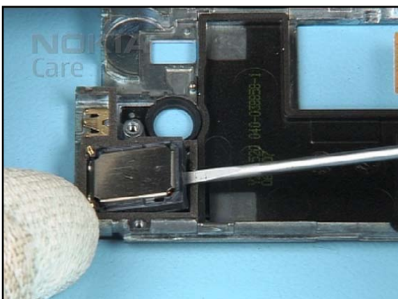
35. Carefully remove the IHF SPEAKER.
