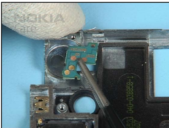
34. Discard the FLASH BOARD ASSEMBLY and also ensure that no adhesive remains.
