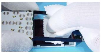
Take a clean cloth and press the *LCD* from the *LCD Frame*.
