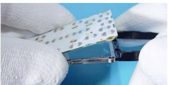
Bend the frame a bit, shift the UI Board Module to the right and then pull it up.
