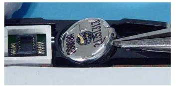
The Speaker is attached with double-sided adhesive Foam Tape. Always use new tape when mounting the *Speaker*.
