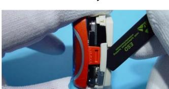
Unlock the top guidance to remove the A-Cover.
