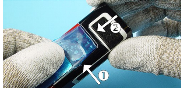
4.) First shift the Slide Cover as far as it will go and then remove it from its guide.
