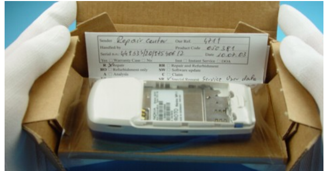
Fold the swap carton as shown in Spare Parts SB-004.
