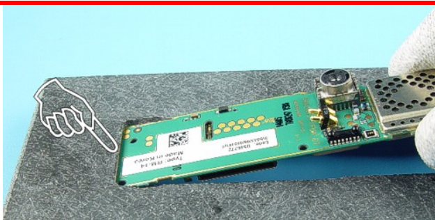
25.) Put the Engine Module into the soldering jig.
