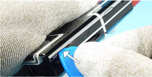
5.) Place SRT-6 between the A-Cover and B-Cover and shift it along the edge. Use always a new A-Cover and a new B-Cover when reassembling.
