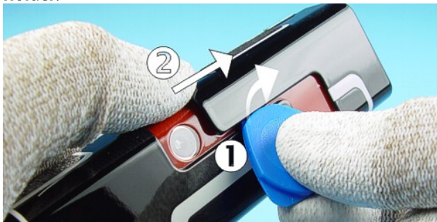
3.) Use the SRT-6 as a lever to remove the Slide Cover.
