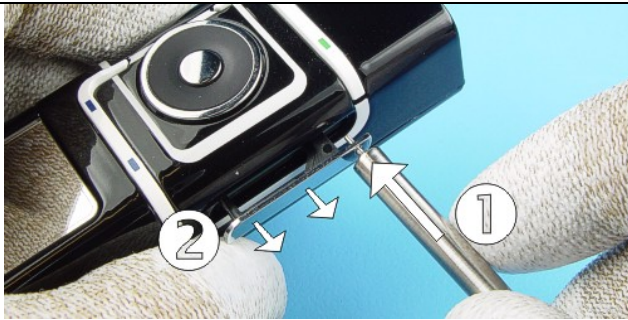
1.) Use the SIM Tray Release Tool to open the SIM Holder.
