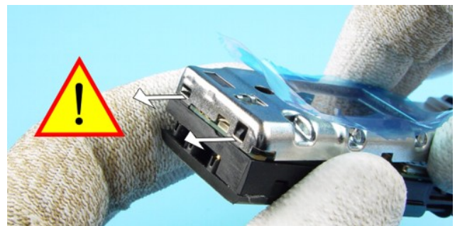
20.) Move the C-Cover Assy a bit to the left as shown in the picture.
