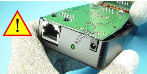
5.) Note the right position of the LED when assembling the Flash Adapter.
