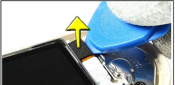
10. Carefully unlock the BOARD TO BOARD CONNECTOR .
