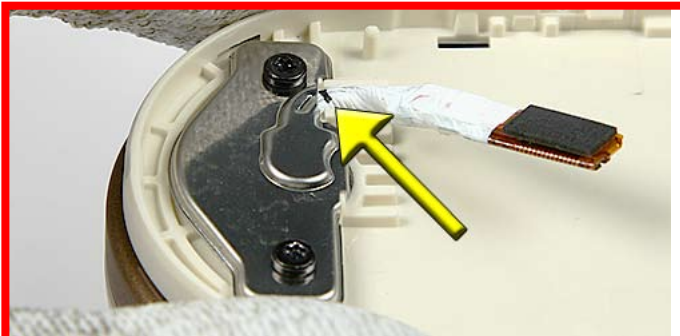
17. For Assembly only: Pay attention to the right length of the COAX CABLE and place the marking at the edge of the SCREWING PLATE .
