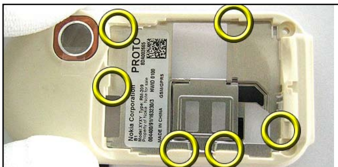
33. There are six clips, holding the LABEL COVER into the D-COVER.
