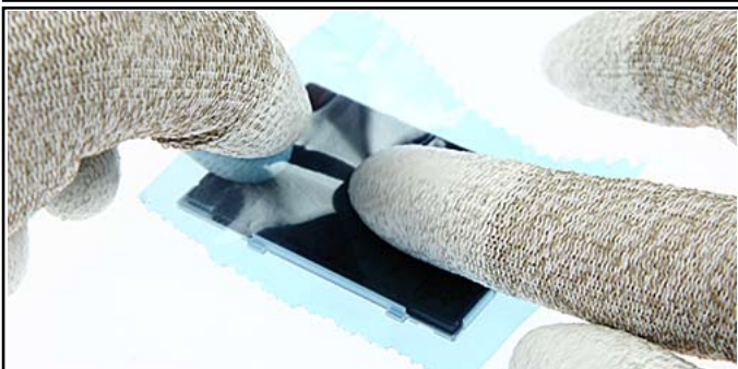
15. To avoid dust and scratches, protect the LCD with a plastic film.
