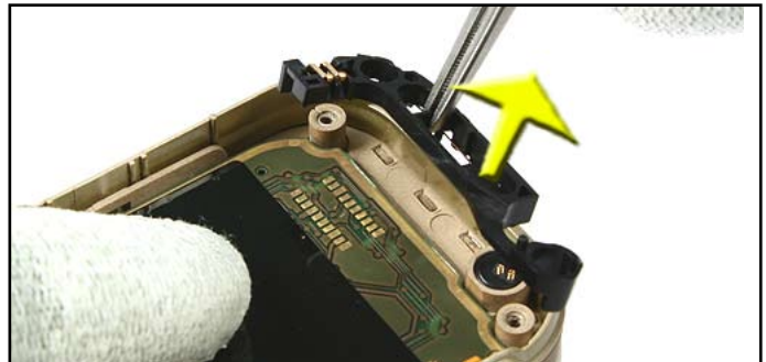
26. Remove the BLUETOOTH ANTENNA with tweezers.
