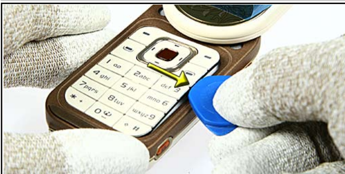
3. If you need to change the KEYMAT , it is also possible at a closed LOWER BLOCK . Remove the KEYMAT starting exactly from the point shown.
