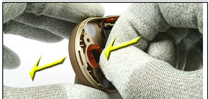
30. Fit the COAX CABLE to the hole to remove the C-COVER ASSY completely from the UPPER BLOCK .
