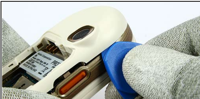
9. Use the SRT-6 to open the snaps of the D-COVER ASSY at the right side . Then ...
