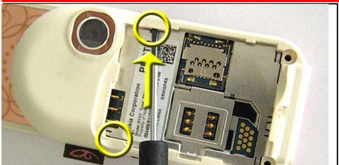
8. Open the middle snaps of the D-COVER , using a slotted screwdriver.
