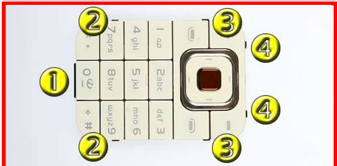
4. For assembly only: When assembling, start placing the KEYMAT at button "0" and move forward to the upper side.
