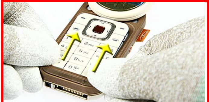
6. For assembly only: Be sure to have all clips locked properly.
