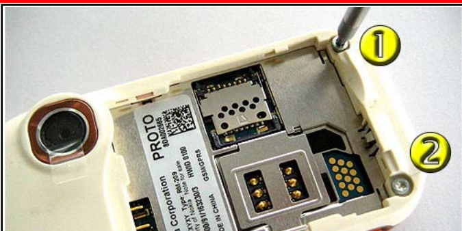
7. Open the two Torx Plus® size 6 screw in the following order. For assembly use the reverse order and apply a torque of 25 Ncm +/- 2Ncm.
