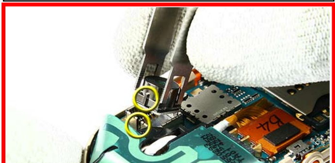
16. For assembly only: Take care of the right positioning of the CAMERA MODULE .
