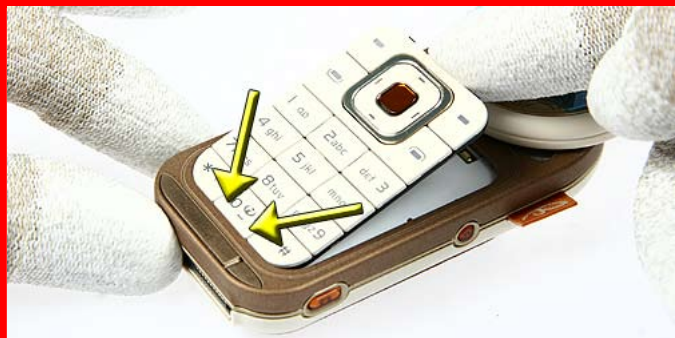
5. For assembly only: Start placing the KEYMAT at the marked positions.
