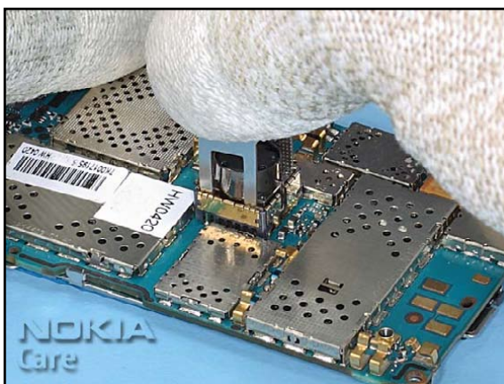
24. Unlock and remove the CAMERA MODULE.
