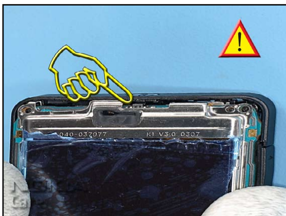
9. Avoid damaging the switch when inserting the ENGINE MODULE into the B-COVER.
