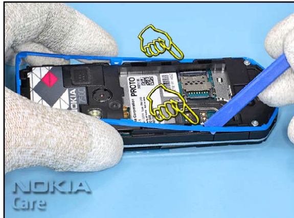
8. Unlock the other clips of the BACK TRIM with the SS-93.
