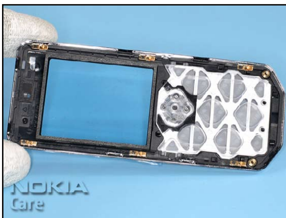
10. Ensure that all spring contacts are in a good condition before fitting the A-COVER.
