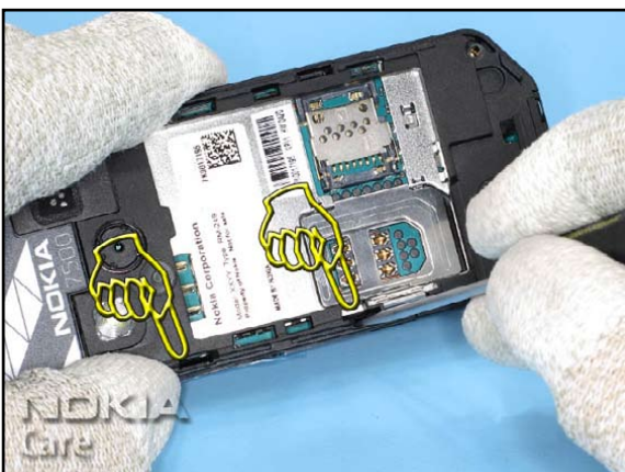
11. Open the clips starting at the shown side.
