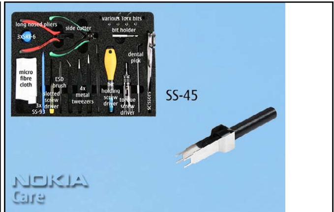
2. You will need the Nokia Standard Toolkit version 2 as well as the camera removal tool SS-45. Also refer to the General Mechanical Guideline Video for additional hints about the tools and component handling.
