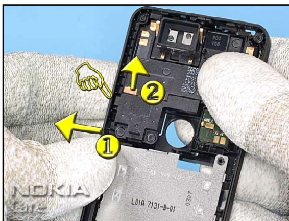
26. To remove the ANTENNA ASSY first unlock the clip on the left side...
