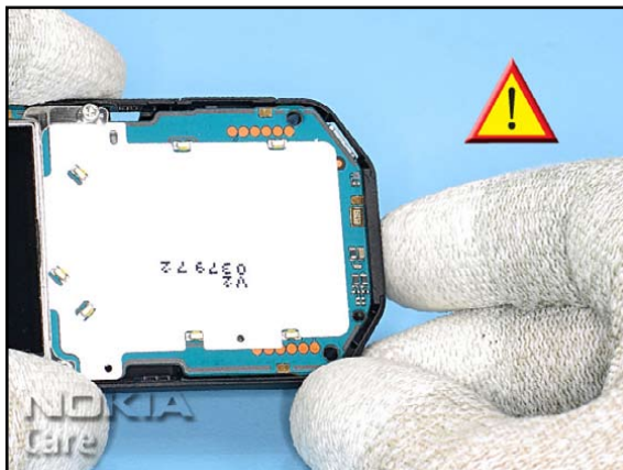
14. Take care of the electronic components on the ENGINE MODULE.
