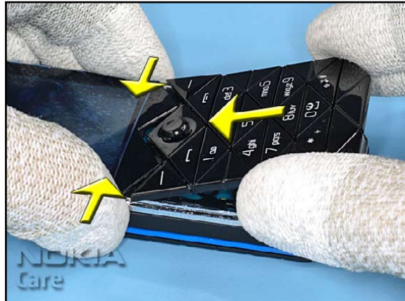
14. Squeeze the A-COVER a bit and gently fit the KEYPAD. Secure it by pressing it into the A-COVER.
