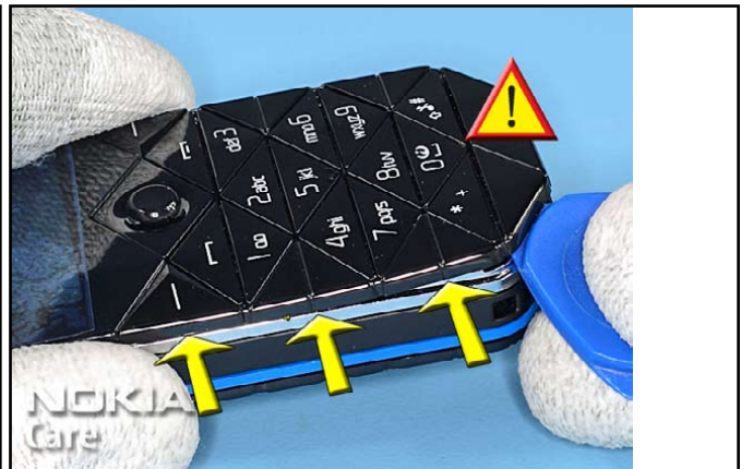
4. Place the SRT-6 between the A-COVER ASSY and the KEYPAD and gently unlock the clips starting at the shown side.
