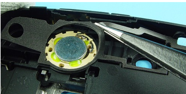
23.) For Side Key Assy removal lift up the IHF Backvolume Gasket first.
