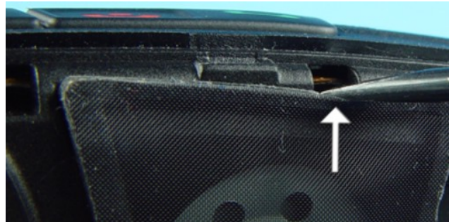
10.) Prevent damaging the IHF Frontvolume Gasket when releasing the second sidekey clip.
