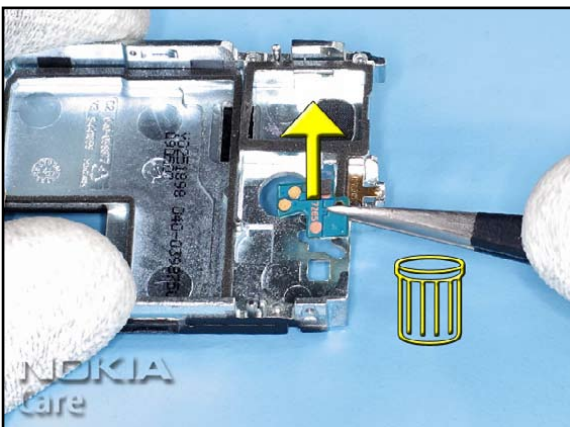
29. Discard the FLASH BOARD ASSEMBLY and also ensure that no adhesive remains.
