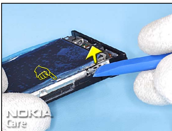
12. The DISPLAY BACK PLATE and the PWB are fixed with the adhesive together. First lift the DISPLAY BACK PLATE beginning at the shown side paying attention to the snap.
