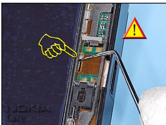
11. Unlock the DISPLAY BACK PLATE with the dental pick.
