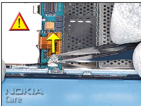
21. Carefully open the coax connector with tweezers.
