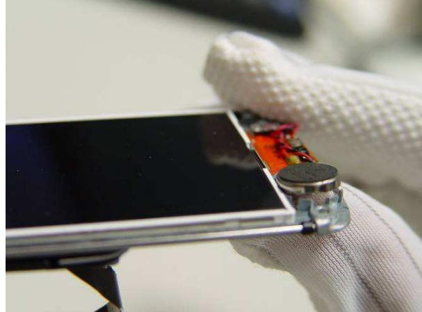
26. Use hands to push bottom of vibrator and pull upward to remove it from the slider module.
