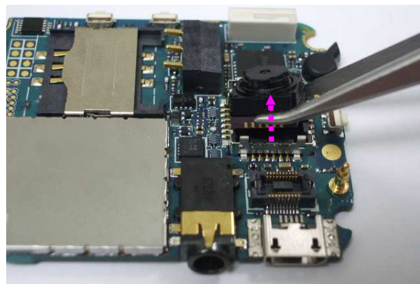
18. Use tweezers to clip camera module and pull upward to release it from the main board.
