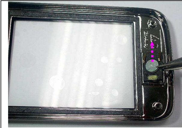
31. Use tweezers to clip the receiver and pull upward to remove it from A - cover.
