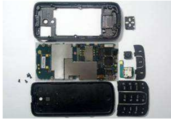
20. Piece parts list of D-cover assembly.
