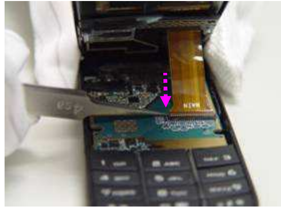
8. Use tweezers to clip FPC connector and pull upward to release FPC from the main board.
