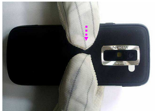
24. Press Battery-Cover on D-Cover peripherally.
