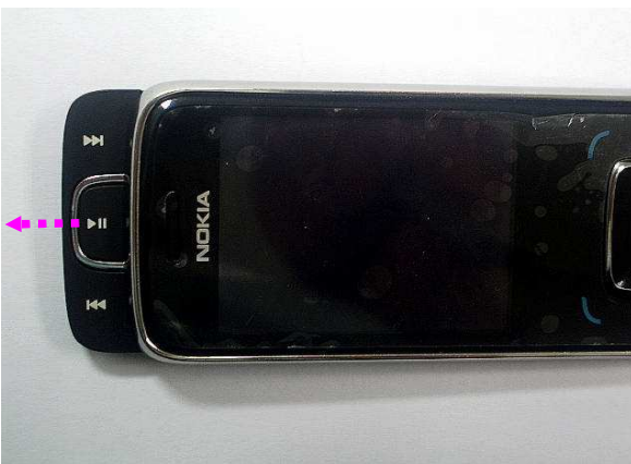
9. Pull left to remove the music key pad from A-cover assembly.
