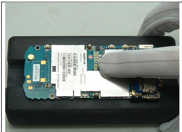
5. Press firmly on the PWB to ensure correct bonding of the dome sheet.
