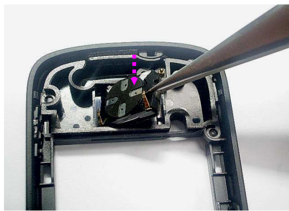
14. Use tweezers to clip speaker and put it into the concave hole of D-cover.
