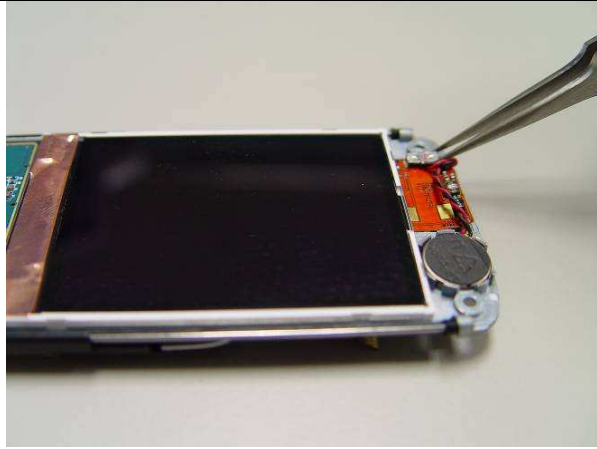
8. Use tweezers to clip connector of vibrator and put it downward to insert into FPC.
