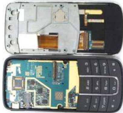
10. Open the A-cover assembly from D-cover assembly.
