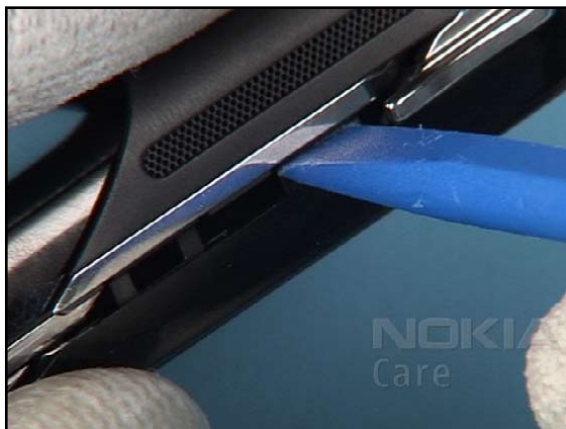
38. Use the SS-93 for bending the latches slightly in order to prevent destroying the plastic clips.
