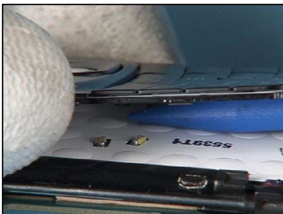
40. Use the SS-93 for bending the keypad. Mind the components underneath.
