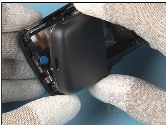
11. Flip over the CAMERA COVER ASSEMBLY DECORATED in order to release the clips on the opposite side. The cover can be removed now.
