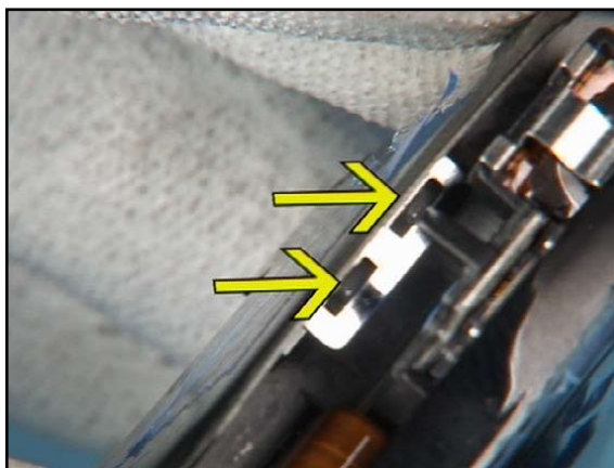
32. Place the CAMERA BEZEL ASSEMBLY, beginning from the top. Mind the hooks.
