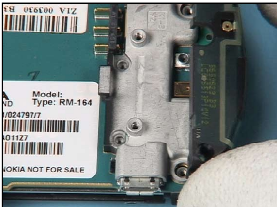
18. Remove the ANTENNA MOD CDMA. The clips of the KEYPAD COVER GUSSET will be released.
