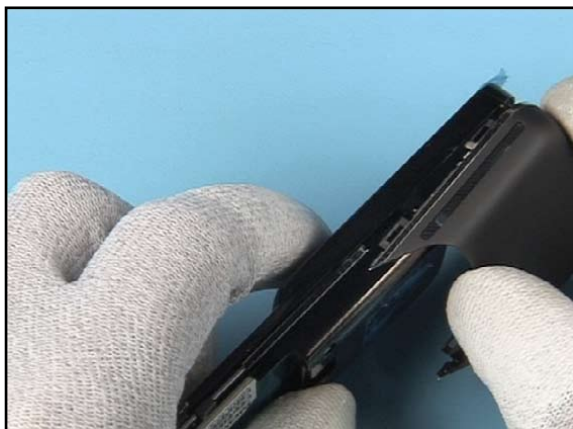
37. Insert the metal snaps of the CAMERA COVER ASSEMBLY DECORATE into their places.
