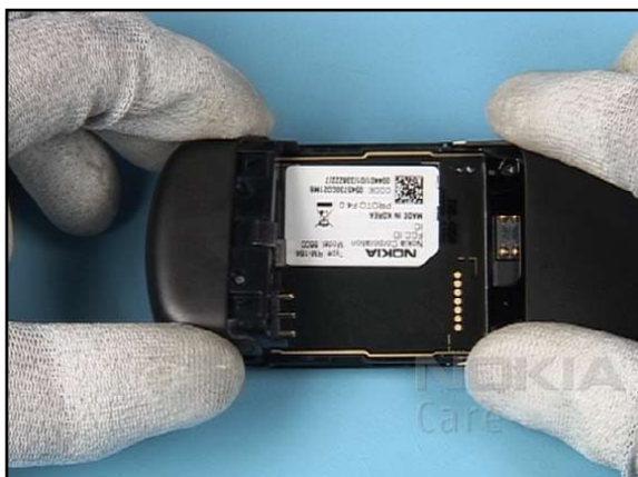
45. Place the ANTENNA COVER ASSEMBLY, beginning at the connector side. Click the snaps into their places.
