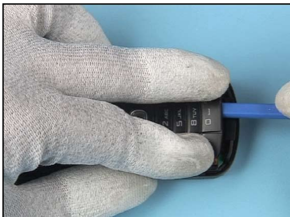
41. Push down the BLACK KEYPAD now while removing the SS-93 carefully. The KEYPAD should snap in place properly.
