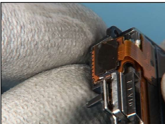
11. Close the connector of the LCD.
