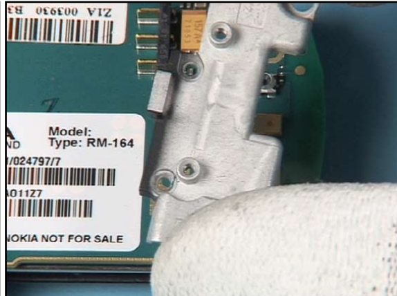
20. Lift up the RF SHIELD PAINTED.
