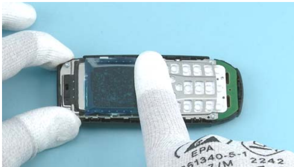
9) Protect the LCD with protective film.
