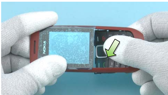
11) Press out the KEYMAT ASSEMBLY from the A-COVER ASSEMBLY as shown.
