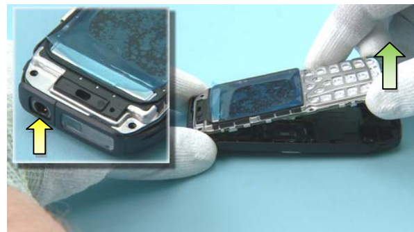
16) Lift up the bottom end of the LIGHT SWAP PACKAGE to release the AV jack.
