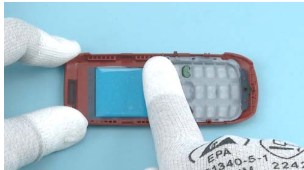
10) Also protect the other side of the A-COVER ASSEMBLY window with protective film.
