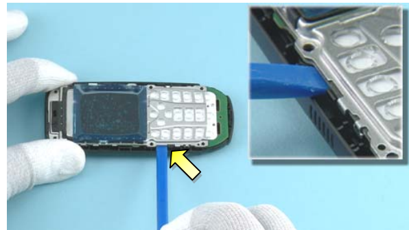
14) Lever out the LIGHT SWAP PACKAGE with the SS-93. Start from the left side.
