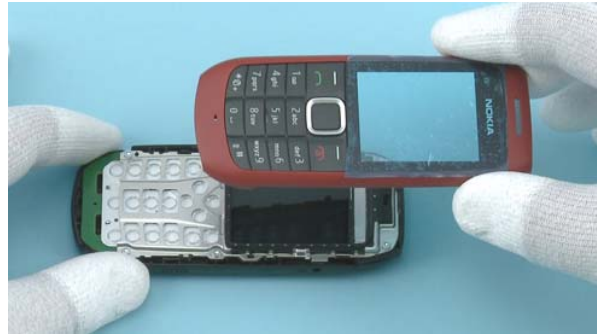
8) Remove the A-COVER ASSEMBLY.
