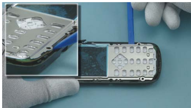
16) Use the SS-93 to release the shown side of the ENGINE BOARD.
