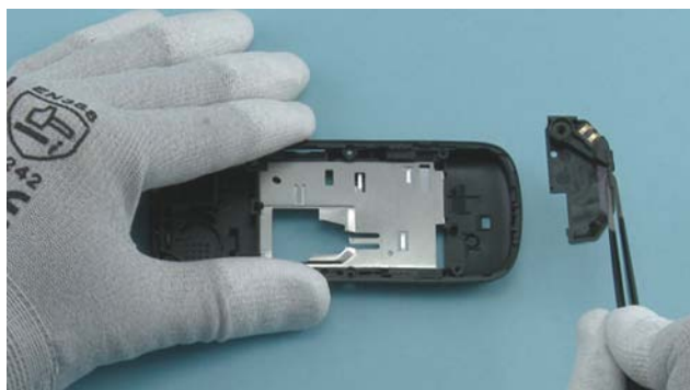
25) Remove the ANTENNA MODULE with the tweezers.
