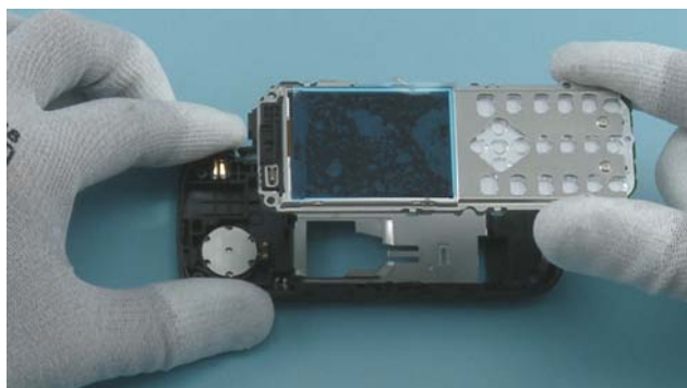
19) Remove the ENGINE BOARD.
