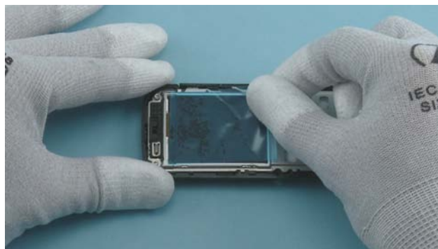
10) Protect the DISPLAY with the protective film.
