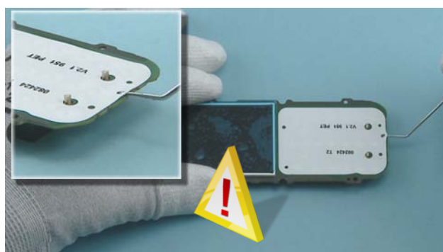
30) Use the dental tool to release the DOMESHEET. Be careful not to injure yourself with the sharp end of the dental tool!
