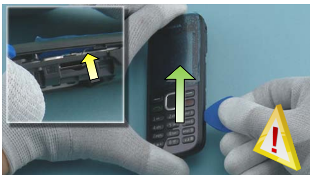
7) Release the A-COVER side from the D-COVER by sliding the SRT-6 to direction shown. Be careful not to damage the shown pin.
