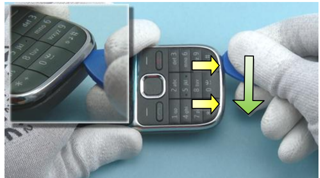
8) Slide the SRT-6 to the direction shown to release the clips on the bottom side of the device.
