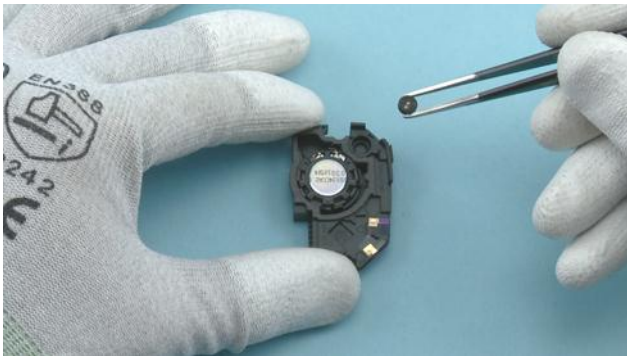
31) Remove the Microphone with the tweezers.
