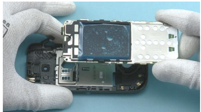
18) Lift up the ENGINE BOARD.
