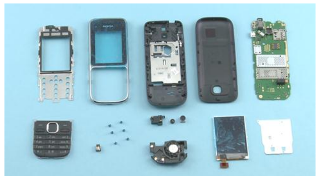
36) The Nokia C2-01 disassembly is now complete.
