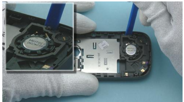
28) Release the ANTENNA ASSEMBLY with the SS-93.
