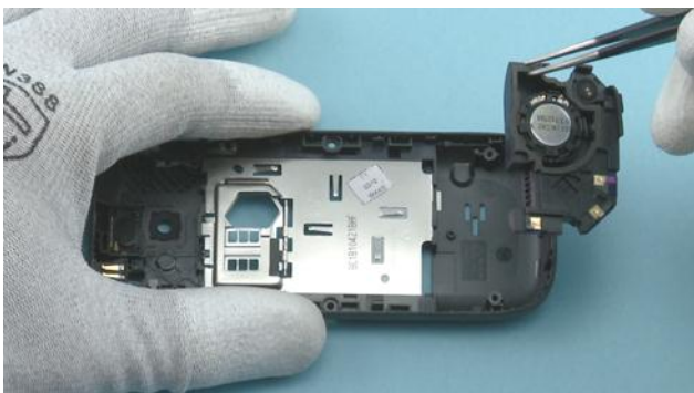
29) Remove the ANTENNA ASSEMBLY with the tweezers.
