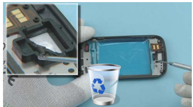
30) Use the dental tool to remove the EARPIECE GASKET. Do not use it again. Discard it.
