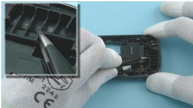
19) Insert the tweezers underneath the ANTENNA MODULE to lift it up and remove it.
