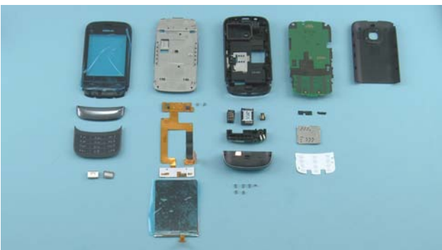
47) The Nokia C2-03 disassembly is now complete.
