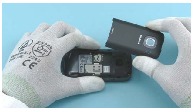
5) Remove the BATTERY COVER.
