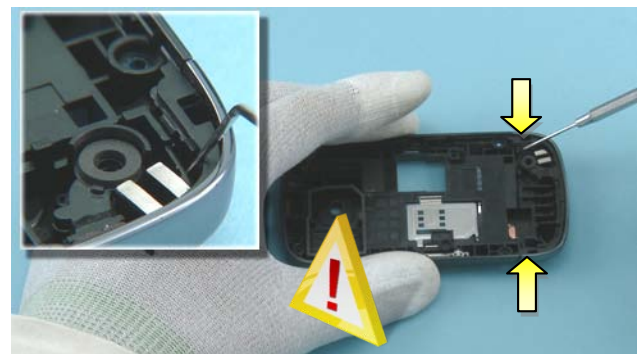
18) Use the dental tool to lift up both sides of the ANTENNA MODULE. Be careful not to injure yourself or any nearby components with the sharp end of the dental tool.
