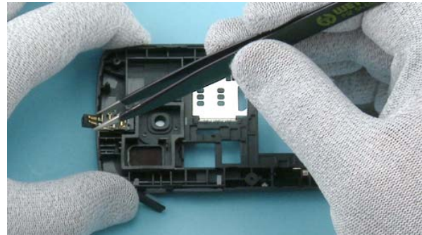
24) Remove the DC JACK with the tweezers.
