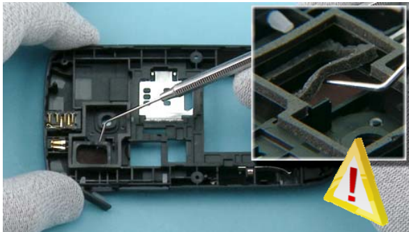
21) Lift up the SPEAKER GASKET with the dental tool. Be aware of the sharp point of the dental tool – be careful not to injure yourself!
