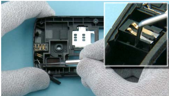
23) Use the dental tool to release the DC JACK.
