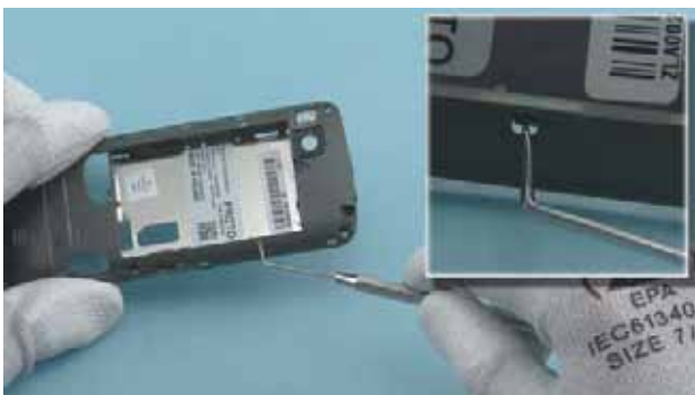
53) Detach the third clip of the METAL INLAY with the dental tool as shown. The METAL INLAY can now be removed.
