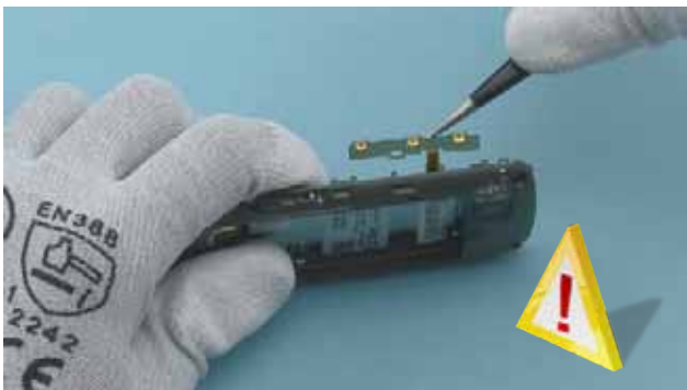
37) Pull the SIDE-KEY PWB out with the tweezers. Do NOT try to detach it from the ENGINE BOARD!
