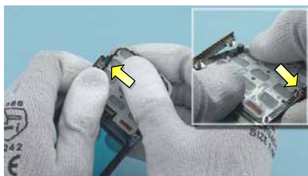
18) Push the corner of the KEYMAT as shown to detach the clip holding it. Release also the clip on the other corner. Pull out the KEYMAT and remove it.
