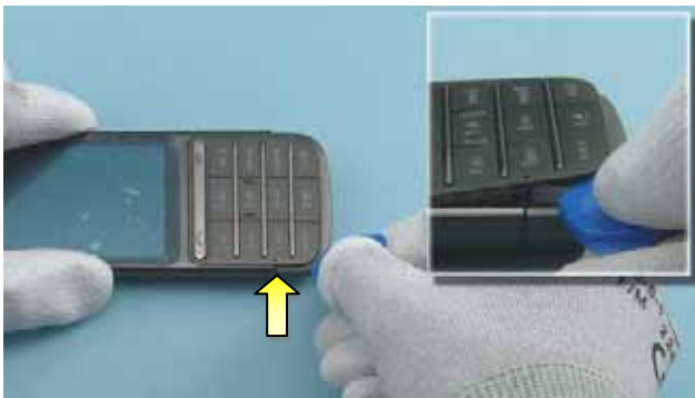
9) Release the KEYMAT clip with the SRT-6 as shown.
