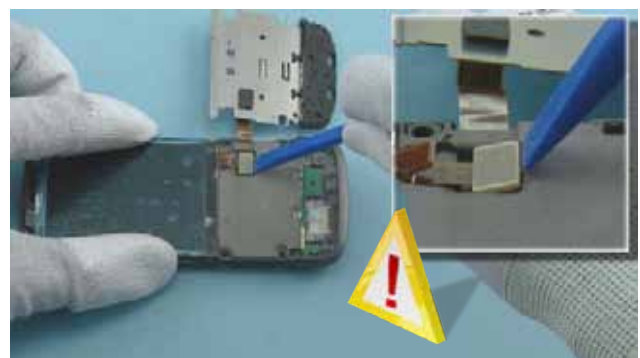
24) Disconnect the DISPLAY connector carefully with the SS-93. Be careful not to damage the connector!
