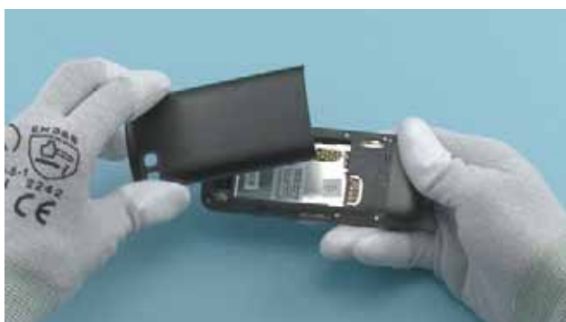
5) Remove the BATTERY COVER. If there is a battery inserted, remove it also.
