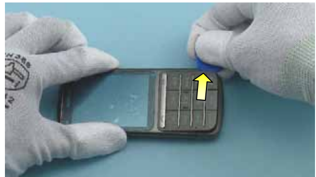
10) Release also the clip on the other side of the KEYMAT.
