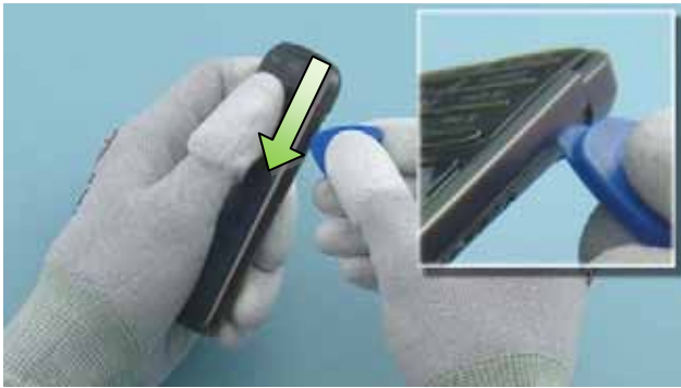
7) To detach the A-COVER, insert the SRT-6 to the place shown, and slide it along the edge.
