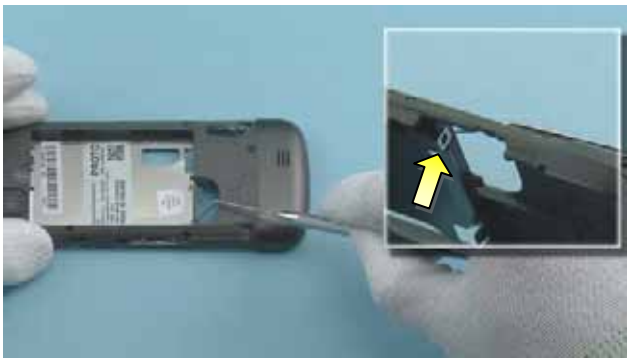
51) Detach the first clip of the METAL INLAY with the dental tool as shown.
