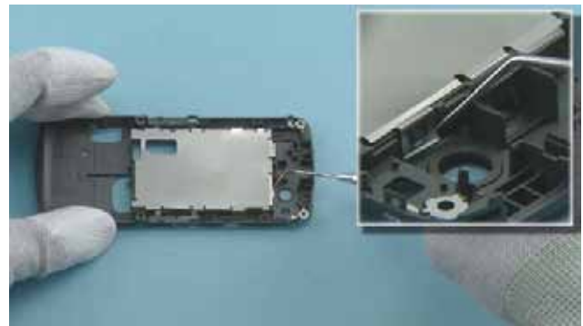
52) Detach the second clip of the METAL INLAY with the dental tool as shown.
