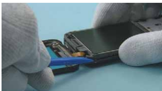
15) Use the SS-93 to detach the top end of the DISPLAY CARRIER.
