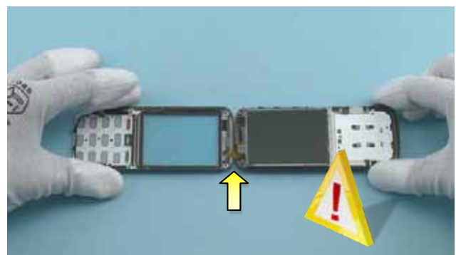
12) Turn carefully the A-COVER as shown. Be careful not to damage the flex while turning the A-COVER.
