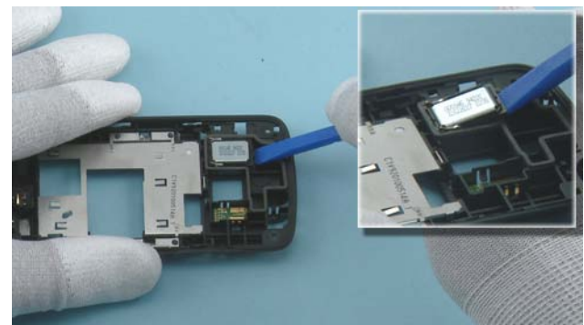
36) Use the SS-93 to lever up the IHF SPEAKER.
