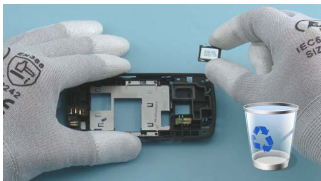
37) Remove the IHF SPEAKER. Do not use it again. Discard it.
