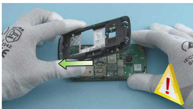
13) Remove the B-COVER to the direction shown, so that the USB connector is not damaged.
