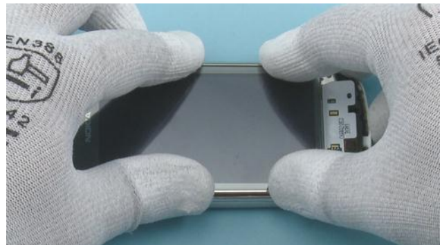
51) Place the A-COVER as shown and make sure that the A-COVER flex does not go between the edges of the A-COVER and the B-COVER.
