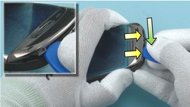
7) Slide the SRT-6 to direction shown to release the A-COVER CHIN clips.
