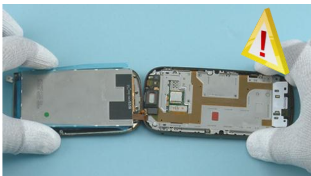
19) While turning the DISPLAY over, be careful not to damage the DISPLAY flex.
