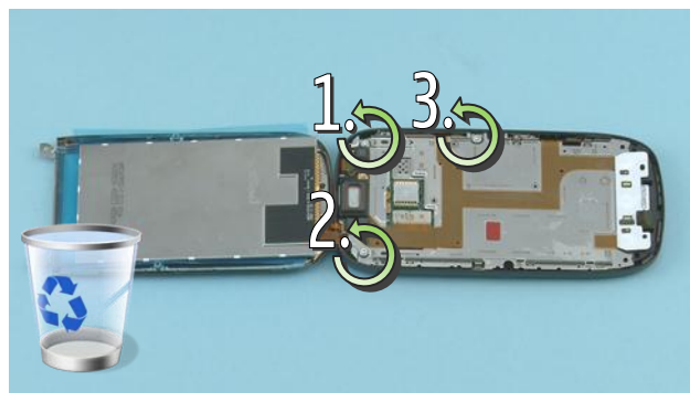
20) Unscrew the three TORX+ size 6 screws in the order shown. Do not use them again. Discard them.
