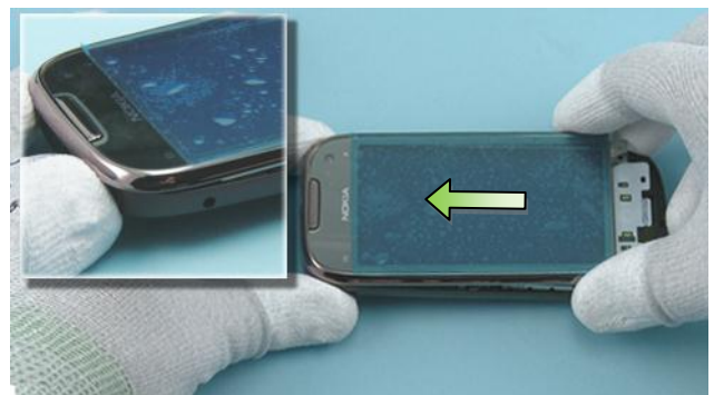
12) Release the A-COVER by sliding it very gently to the direction shown.
