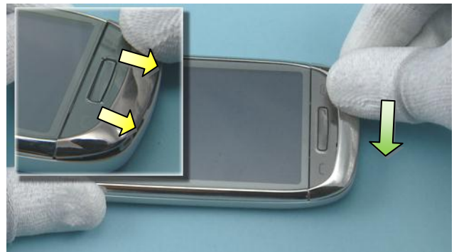
57) Press the A-COVER CHIN from the top to lock the two clips on the bottom end.
