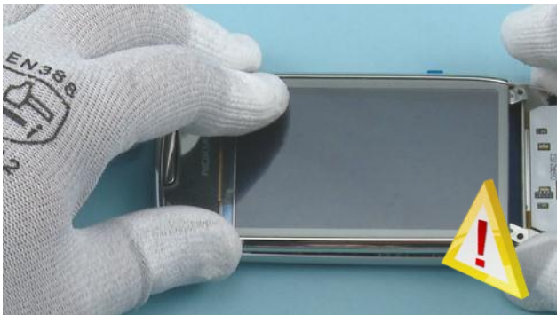
50) Turn over the A-COVER. Be careful not to damage the flex!
