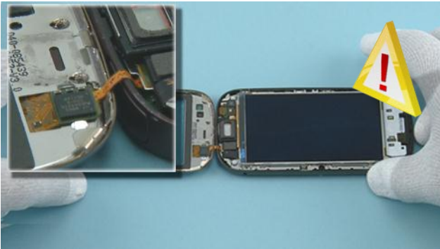
13) Turn the A-COVER around carefully. Be careful not to damage the flex.
