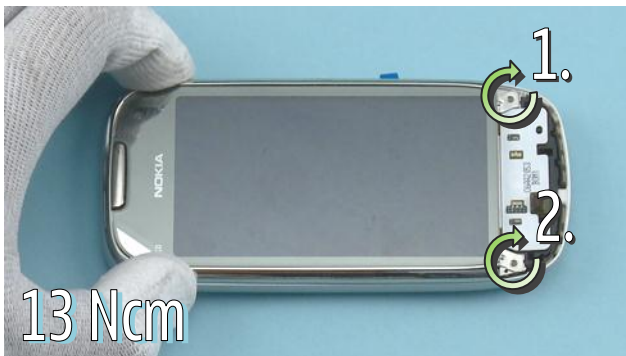
54) Tighten the two TORX + size 6 screws to the torque of 13 Ncm in the order shown.
