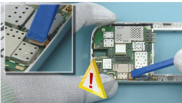
16) Connect the SIM CARD READER connector with the SS-93. Be careful not to damage the connector or components nearby!
