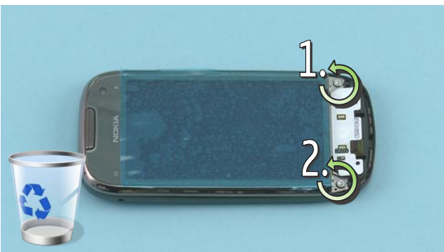
11) Unscrew the two TORX+ size 6 screws in the order shown. Do not use them again. Discard them.
