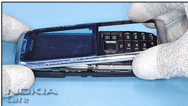
5. Remove the A-COVER ASSY.
