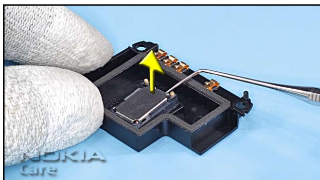
20. Remove the IHF SPEAKER with the dental pick.
