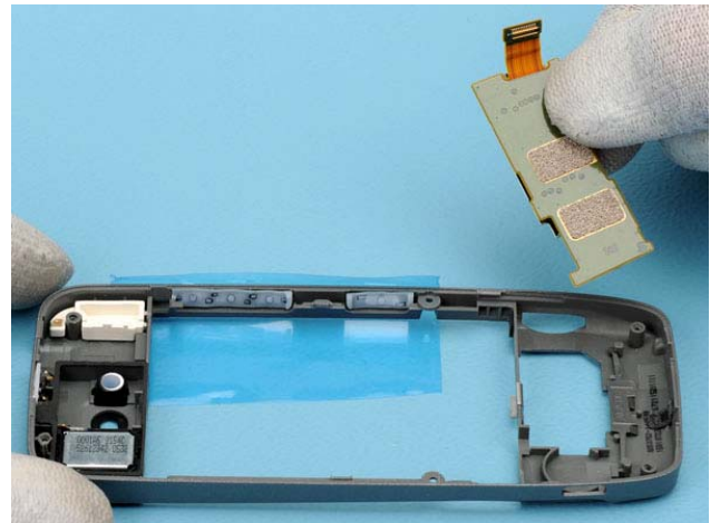
Remove the CARD READER MODULE from the B-COVER.
