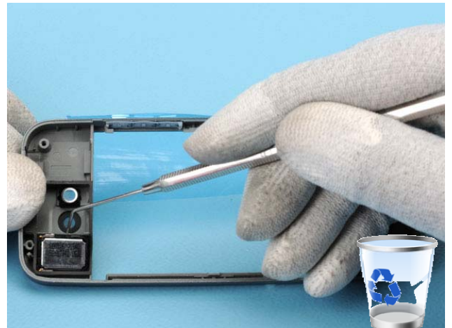
Lift up the IHF SPEAKER using a dental tool.
