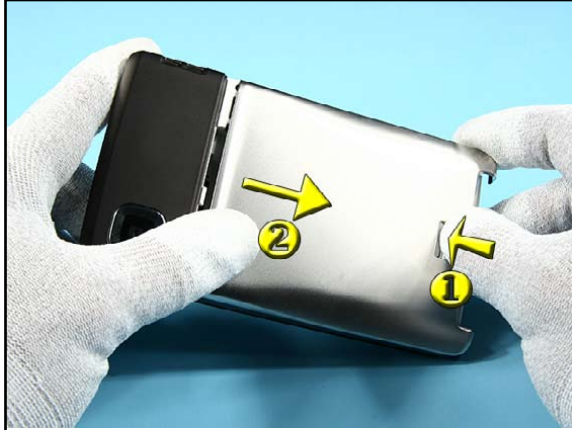
2. Push the BATTERY RELEASE BUTTON and remove the BATTERY COVER.
