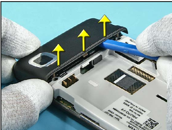
5. Then Gently, lift the CAMERA LID with the SS-93 and remove it.
