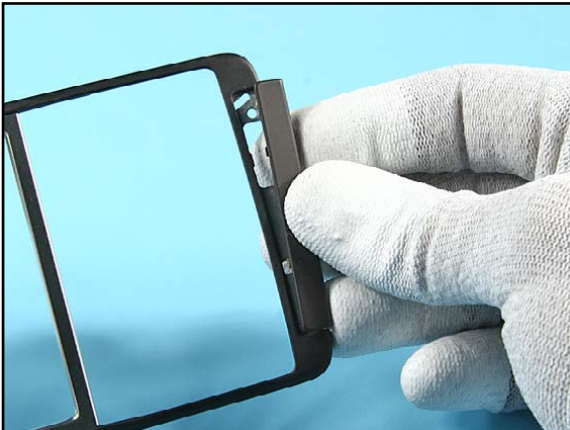
9. If needed, carefully unlock and remove the OPERATOR LOGO.
