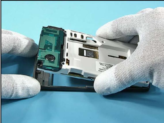
7. Remove the assemblies from the A-COVER.
