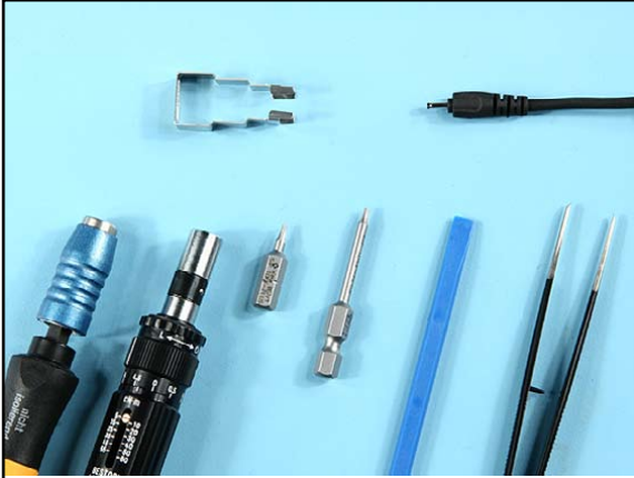
1. Needed tools: a Torx driver, a torque driver, a Torx plus size 4 bit, a Torx plus size 6 bit, the SS-93 opening tool, metal tweezers, the SS-102 camera removal tool and a DC-plug.
