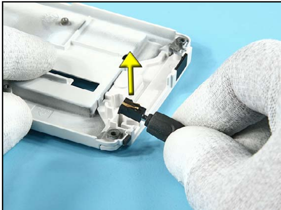
18. Use the DC-PLUG to remove the DC-JACK.
