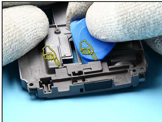
26. Unlock the both snaps of the CONNECTOR HOUSING INCL. IRDA WINDOW...
