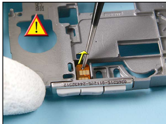
24. Unlock the SIDE BUTTON MODULE ASSY...
