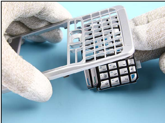
15. Separate the KEYMAT from the A-COVER ASSY.
