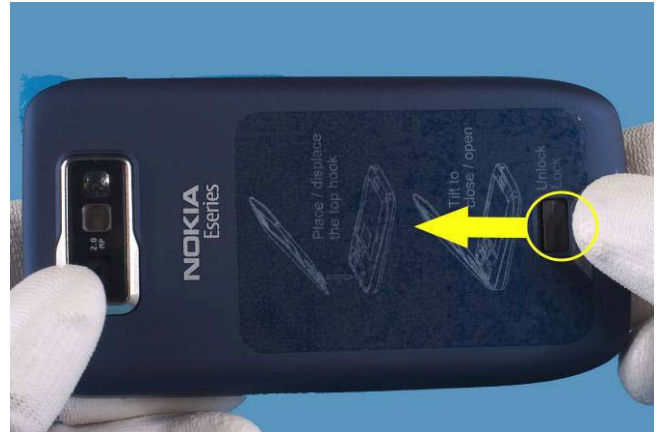
2) Unlock the release button in the direction as shown.
