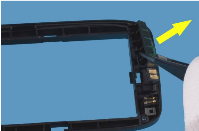
23) ANTENNA MODULE can be taken away.
