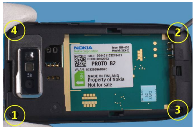
4) Remove the four TORX 6+ screws using a screwdriver. The screws are reusable.
