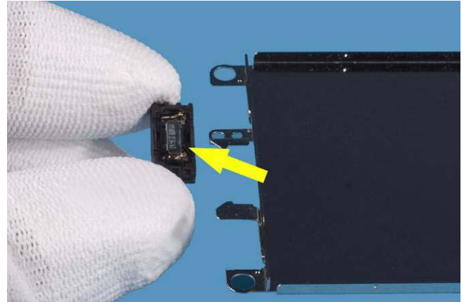
16) Pull out the EARPIECE RUBBER HOUSING inclusive EARPIECE STOUT as shown.
