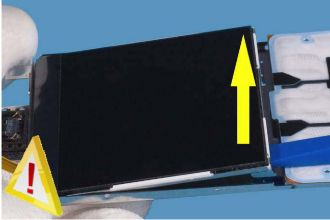
13) Use SS-93 tool to detach the LCD carefully.
