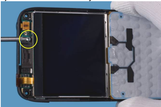
9) Unscrew the TORX 6+ screw and remove it. The screw can be reused.
