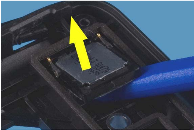
25) Lift up the IHF SPEAKER DONAU with SS-93 tool in order to remove it.
