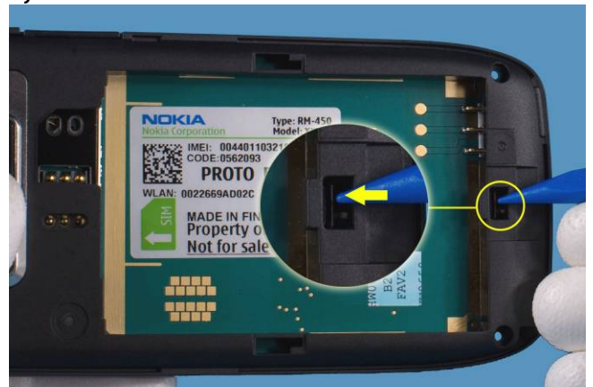
10) Use the peak side of SS-93 tool to detach the clip of the ATO-FRAME ASSY on the bottom side of the phone.
