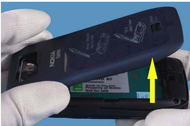
3) Lift up and remove BATTERY COVER ASSY .
