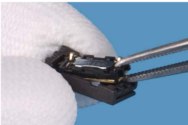
17) Remove EARPIECE STOUT with tweezers.
