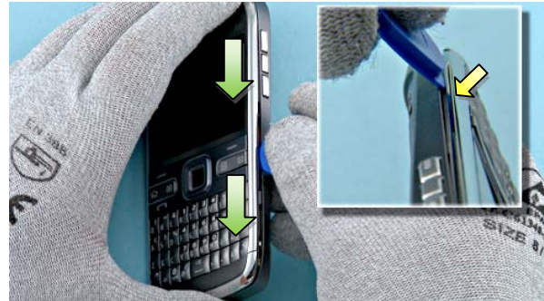
6) Using the same procedure release also the clip on opposite side of the A-COVER.
