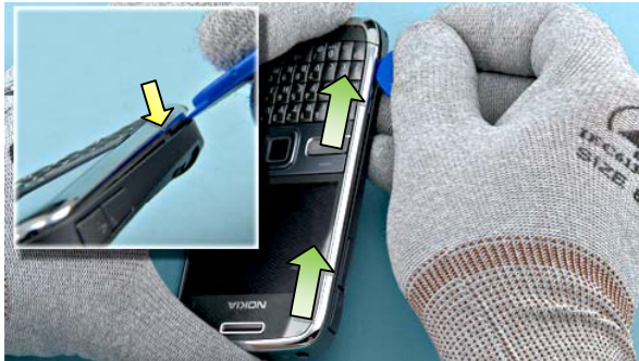
4) Insert the SRT-6 between the A-COVER ASSEMBLY and the B-COVER ASSEMBLY. Slide it from top to bottom to release the clip holding the A-COVER ASSEMBLY.
