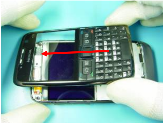
7. Remove the A COVER as shown.
