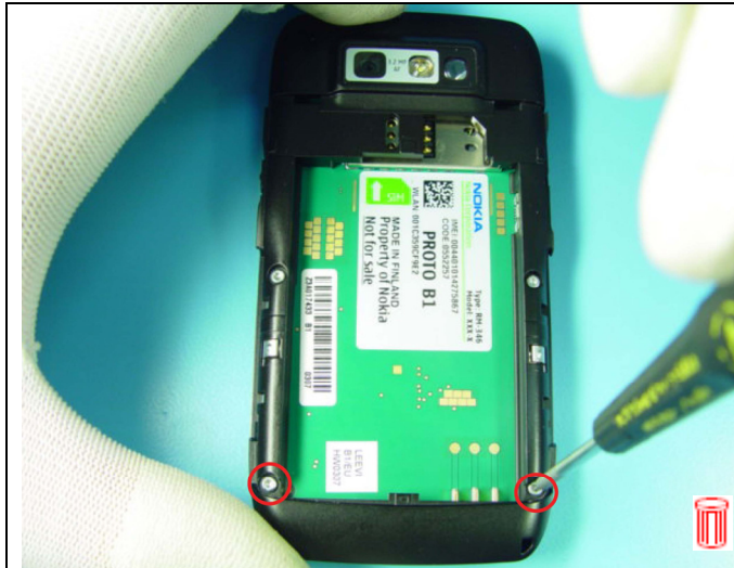
1. Remove the two screws T4.
