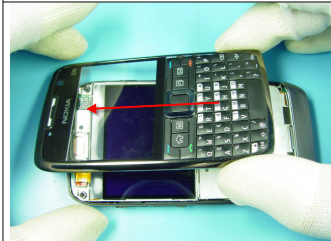
5. Remove the A COVER as shown.
