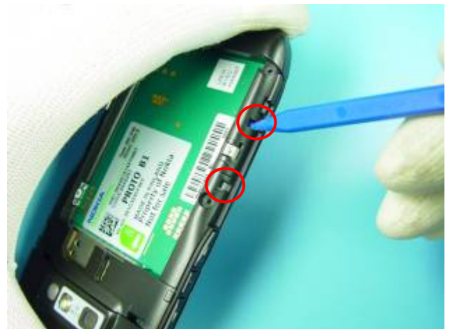
4. Open the two clips of the A-COVER.
