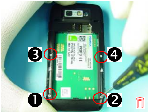
3. Unscrew the four screws T4+.
