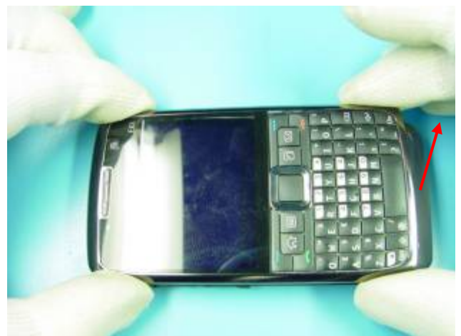
6. Lift up the A COVER on the bottom side.
