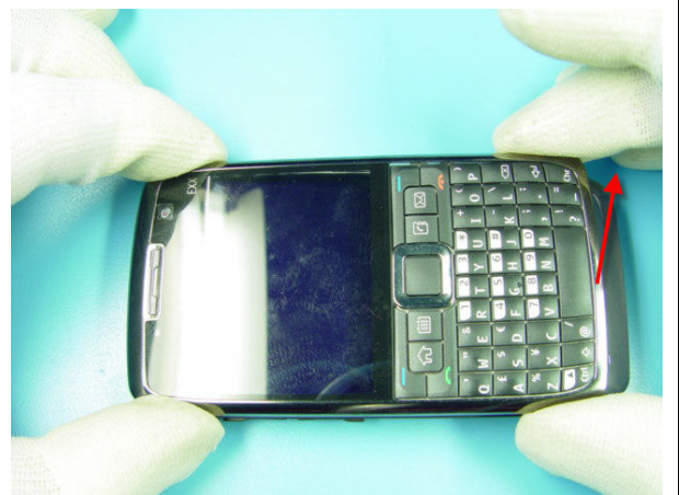
4. Lift up the A COVER on the bottom side.
