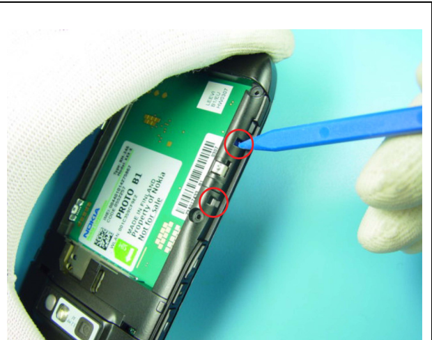
2. Open the A COVER's snaps (2 pcs + 2 pcs) from the B COVER side by lightly lifting with tweezers.
