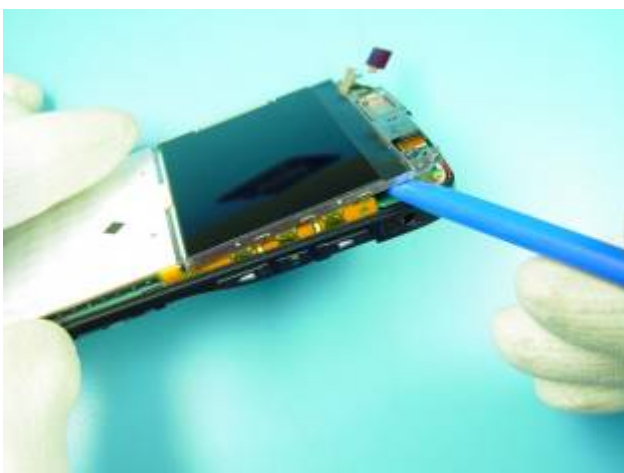
11. Release the shield assy with LCD.
