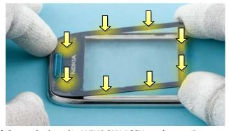
9) Start placing the WINDOW ASSY as shown. Press marked areas to activate the adhesive on the WINDOW ASSY. Maintain the pressure for 5 seconds.
