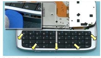
12) Slide the phone open and release the five clips holding the QWERTY KEYMAT using the SRT-6. Release the clip near the space bar first.
