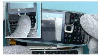
6) Lift up the A-COVER ASSEMBLY. Separate the KEYMAT ASSEMBLY from the A-COVER ASSEMBLY. Remember to protect the LCD with protective film.
