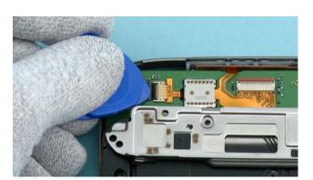
17) Open the AV connector with the SRT-6.
