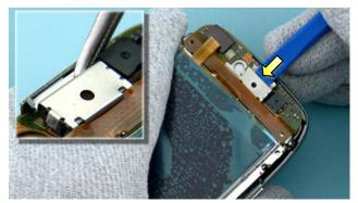
7) Release the EARPIECE HOLDER with the SS-93 and remove it with the tweezers.
