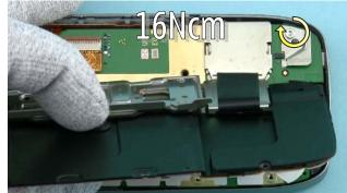
5) Tighten the screw to the torque of 16 Ncm.
