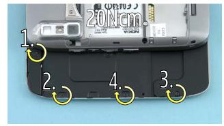
10) Tighten the screws to the torque of 20 Ncm in the order shown.
