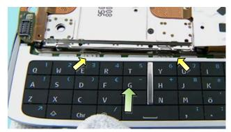
7) When assembling the QWERTY KEYMAT, slide the clips into their gaps. Also make sure that clips in both ends of the QWERTY KEYMAT are correctly aligned.
