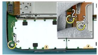
15) Unscrew these three Torx+ size 4 screws. After unscrewing the first screw, close the slide a bit until the two remaining screws become visible.
