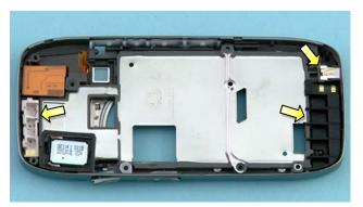
25) Remove the DC JACK, ANTENNA ASSEMBLY, and GPS/BT WLAN ANTENNA with the tweezers.
