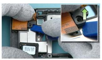
26) To release the AV JACK, slide the SS-93 under the clip and carefully lift it up as shown. Then remove the AV JACK.
