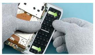
13) After releasing the clips pull the QWERTY KEYMAT in the direction shown.
