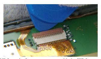
18) Open the Camera connector with the SRT-6.
