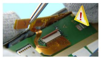
19) Lift up the Camera Flex with the tweezers. Be careful not to damage the flex.
