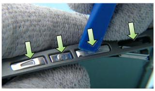
28) Carefully push each button of the SIDE KEY with SS-93 to remove it.
