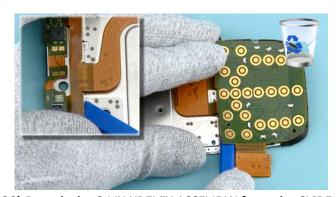
28) Detach the 2 MX UI FLEX ASSEMBLY from the SLIDE MODULE with the SS-93. Discard the 2MX UI FLEX ASSEMBLY, do not use it again.
