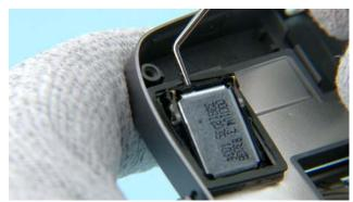
29) Finally use the dental tool to release the IHF SPEAKER and the IHF SPEAKER gasket.
