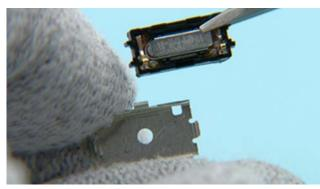
8) Separate the EARPIECE from the EARPIECE HOLDER with the tweezers.
