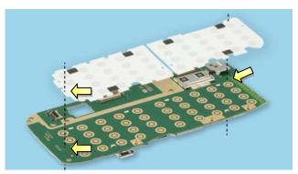
1) When placing the QWERTY DOMESHEET make sure that these holes are aligned.
