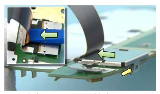
2) First push the DYNAMIC FLEX with the SS-93 into place against the FLEX PLANE as shown. Next, connect the connector to the PWB. Then slide the FLEX PLANE into gap shown and fasten the small clip.
