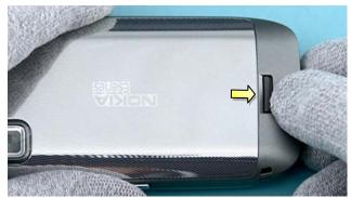
3) To remove the BATTERY COVER ASSY, push the button on the bottom side and then lift up the BATTERY COVER ASSY.
