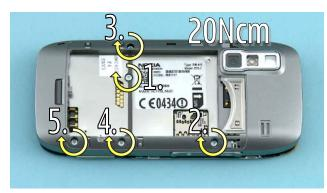
8) Tighten the screws to the torque of 20 Ncm in the order shown.
