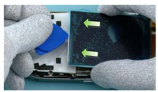
11) Carefully lift up the LCD and push it into direction shown.
