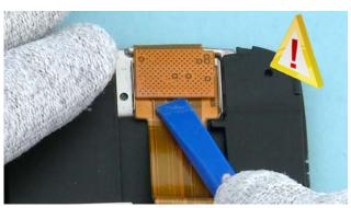
26) Open the connector of the DYNAMIC FLEX and separate it from the SLIDE MODULE. Be careful to not to damage the connector.
