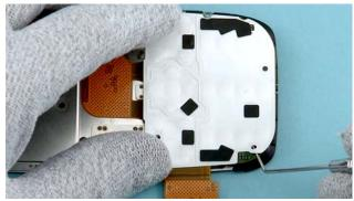
27) Peel off the DOMESHEET using the dental tool.
