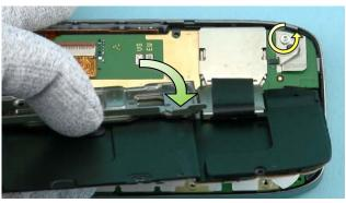
16) Rotate the SLIDE ASSY and unscrew the Torx+ size 4 screw.
