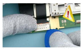
24) Open the DYNAMIC FLEX connector with the SRT-6 and separate the engine board and the SLIDE MODULE. Be careful not to damage the connector.
