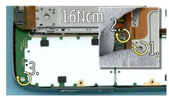
6) Tighten the screws to the torque of 16 Ncm in the order shown.
