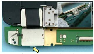
23) Remove the FLEX PLANE from the engine board by opening a small clip with the dental tool.
