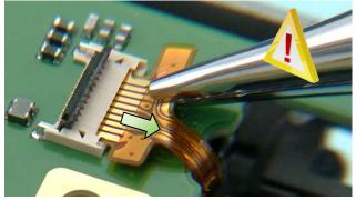
21) Use the pliers to open the AV connector. Be careful not to damage the connector.
