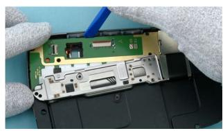
22) Separate the SLIDE MODULE and the engine board from the B-COVER.
