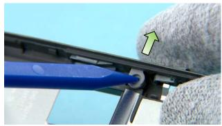
27) Use the sharp end of the SS-93 to push out the USB/SD-DOOR.
