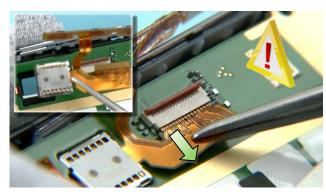
20) Use the tweezers to open the Camera connector. Be careful not to damage the connector. Then remove the Camera Assembly with the tweezers.
