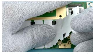
30) Carefully remove the QWERTY DOMESHEET. Make sure that the whole QWERTY DOMESHEET is removed.
