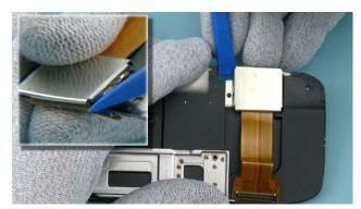
25) Remove the FLEX SLIDER using the SS-93.
