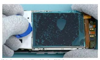
10) Release the LCD with the SRT-6.
