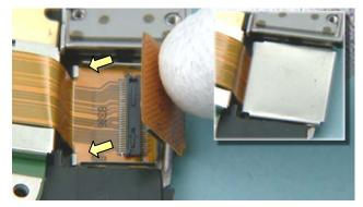
3) When assembling the other end of the DYNAMIC FLEX make sure that the connector goes under the two clips shown. Connect the connector and then press the FLEX SLIDER into correct place so that the small gap is facing the DYNAMIC FLEX.
