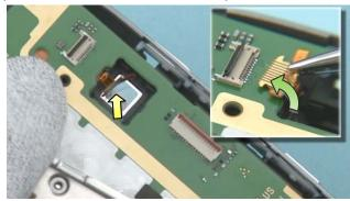
4) When placing the PWB, make sure that the AV-JACK FLEX is properly routed through the camera. Carefully connect the connector with the pliers.
