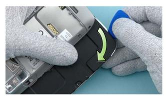
5) Release the A-COVER ASSEMBLY from the SLIDE MODULE using the SRT-6. Start from the bottom end of the phone and continue to the direction shown.
