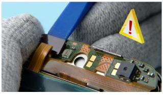
9) Open the LCD connector from the 2 MX UI FLEX ASSEMBLY with the SS-93. Be careful not to damage the connector.
