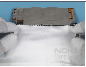
16. It is important to protect the surface with a piece of cloth before continuing. Flip over both parts of the hinge.
