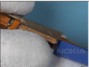
18. Be double carefully while opening these 2 MICROCOAX HARNESS connectors.
