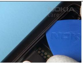
4. Now release the two clips on the side of the assembly.
