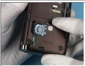
6. Now the ANTENNA COVER can be removed easily.
