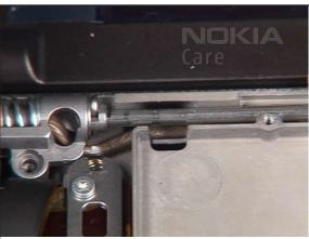
9. Replace the upper assembly. Mind the correct positioning of 10. Note: False placement will destroy the delicate MICROCOAX cables.
