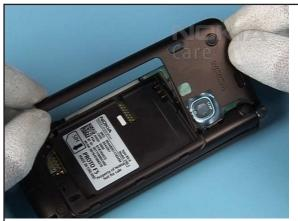
31. Mind the cleanness of the camera and window when replacing the ANTENNA COVER, beginning at the hinge side.
