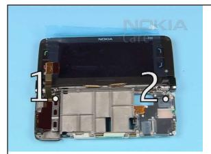
13. Apply the torque to both screws.
