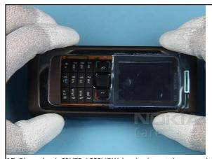
17. Place the A-COVER ASSEMBLY, beginning at the opposite side of the hinge.
