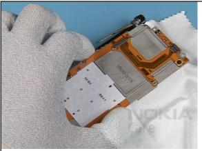
20. Now the CHASSIS ASSEMBLY can be removed.
