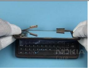
3. Fit the C-COVER. Note the correct alignment to the mounting 4. Flip over the C-COVER ASSEMBLY together with the mounting parts of the hinge.
