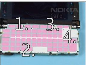
22. Apply the torque to these screws in the order shown.
