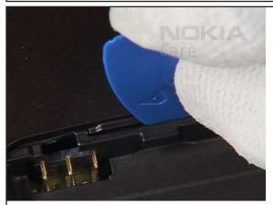
3. Release this clip of the ANTENNA COVER with the SRT-6 first.
