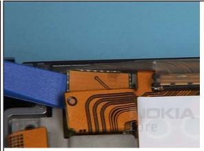
14. Gently lever up the flex connector of the LCD AM 800x352.
