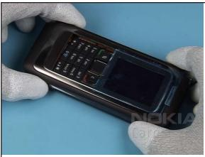
6. Close the assembly again. Lift up the A-COVER at the hinge side. Move it away from the hinge side. Now it can be removed easily.
