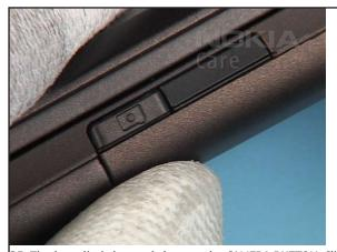
35. The last clip is located close to the CAMERA BUTTON. Click it 36. Replace the BATTERY COVER. into its place slightly.
