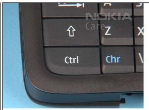
20. Mind the correct positioning of the key mat before going on.
