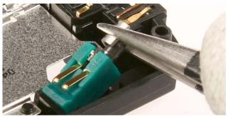
26.) Remove the **Vibra Motor** with tweezers.
