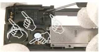
30.) Unlock the 4 plastic clips of the **Antenna Assy** in the area shown.
