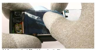
6.) Protect the **LCD** with a plastic film.
