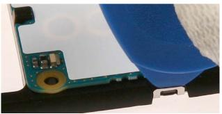
21.) Unlatch the BB shield Assembly first.
