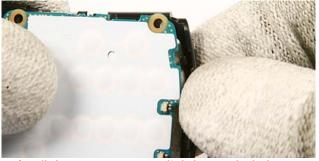
23.) Pull the **UI Frame Assy** slightly to unlock the **UI PWB.**
