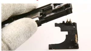
31.) Carefully separate the **Antenna Assy**.
