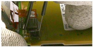
17.) Open the flex connector with the SS-34 flex connector-opening tool. Mind the surrounding components while placing the tool. Now the **UI-Frame Assy** can be removed.
