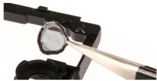
20.) Also remove the **Earpiece Gasket** from its compartment. **Always use a new gasket when reassembling.**
