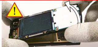
16.) Lift the **UI-frame Assy** from **Chassis Assy**. Mind the still connected flex foil of the **LCD**.
