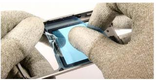
7.) Also protect the inner side window with a film
