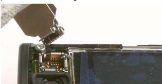
13.) Unlock and remove the **VGA Camera** with the **SS-51** camera removal tool. (N70 only)
