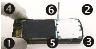
15.) Unscrew the 6 Torx size 6 plus screws in the shown order. For Assembly use the reverse order and the torque of 25 Ncm.
