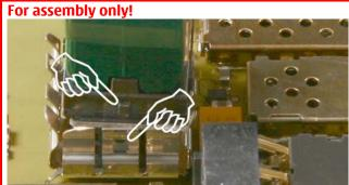
36.) Mind the correct position of the camera while assembling.
