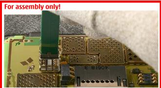
35.) Use the Assembly side of the SS-15 for fitting the Camera Module 2MP into its compartment.
