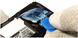
32.) Lever out the Camera Rear Bezel Assy.
