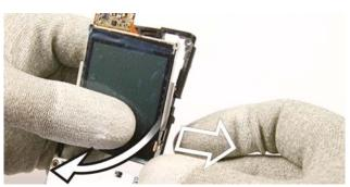
18.) Unlatch each clip of the **LCD** from the **UI Frame Assy** carefully by pulling the **UI Frame Assy** sideward while pushing the LCD forward.
