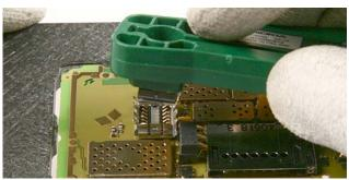
34.) Remove the **Camera Module 2MP** with the SS-15 camera removal tool. Always use the RJ-94 rework jig as support to prevent mechanical stress to the PWB.
