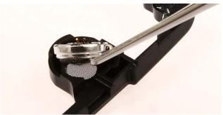
19.) Remove the **Earpiece** with the dental tool
