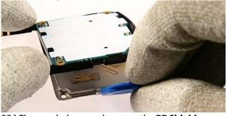
22.) Then push down and remove the **BB Shield Assembly.** The shield can't be reused again, always use a new one.
