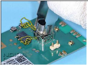
23. Unlock and remove the MAIN CAMERA with the SS-45.
