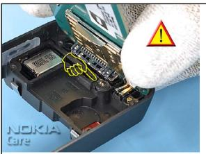
2. Place the ENGINE MODULE into the B-COVER starting on the shown side. Take special care to the spring contacts of the MICROPHONE.
