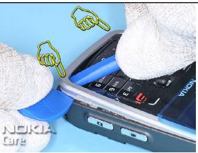
4. Place the SS-93 between the KEYMAT and the edge of the A-COVER and unlock the buttom clip first. Hold the SS-93 in the shown position and unlock the side clip with SRT-6 by pressing it between the A-COVER and the B-COVER. Do the same on the other side.
