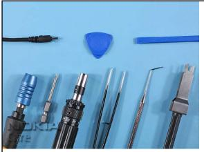
1. Needed tools: A Torx driver, a Torx Plus© size 6 bit, a torque driver, metal tweezers, a dental pick, the SS-45 camera removal tool, a DC plug, the SRT-6 and the SS-93 opening tool.
