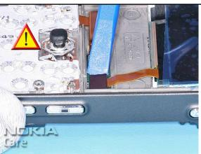
10. ...and disconnect it from the ENGINE MODULE.
