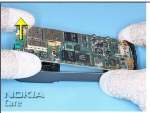
20. Remove the ENGINE MODULE from the B-COVER.
