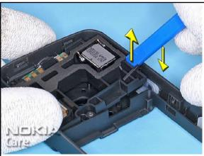
24. Unlock and remove the ANTENNA MODULE ASSEMBLY.
