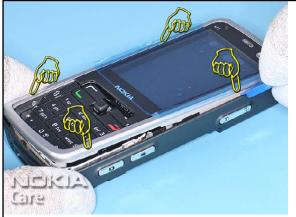
5. Slide the SRT-6 along the marked edges to unlock the snaps. 6. Gently remove the A-COVER from the B-COVER ASSEMBLY.
