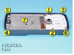
6. First tighten the six screws (1-6) to the torque of 25Ncm, then set the torque driver to the torque of 28Ncm and tighten the last screw.
