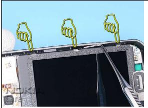
8. Carefully unlock and remove the DISPLAY SHIELD by using the dental tool.
