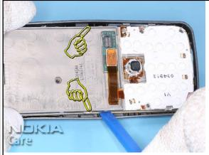
14. The UI FRAME is attached with two snaps to the B-COVER. Unlock the UI FRAME with the SS-93.
