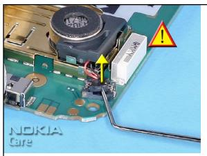
21. Carefully open the VIBRATOR connector.
