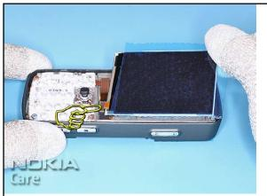
9. Cover the LCD MODULE with a protective film. Gently lift out the LCD MODULE from the UI FRAME...
