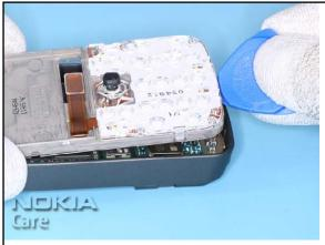
15. Lift the UI FRAME a bit with the SRT-6 and remove it.
