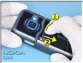
2. Cover all sensitive surfaces with a protective film. Unlock and open the C-COVER ASSEMBLY. Remove the Battery if inserted.
