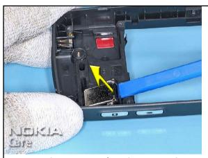
27. Remove the IHF SPEAKER from the B-COVER. The DC-Jack and the MICROPHONE can be removed easily.
