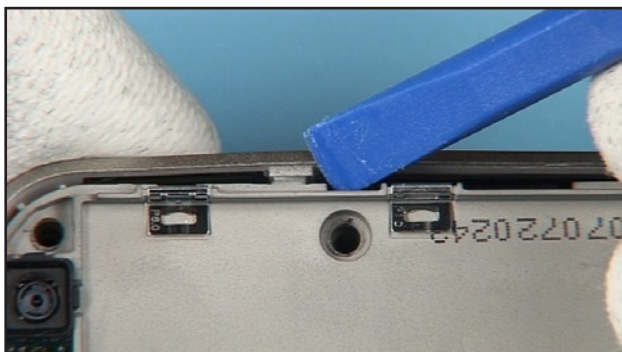
25. Gently pry open the clips of the cover.
