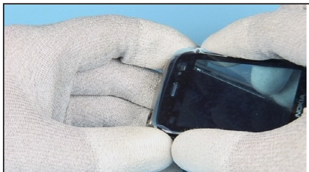
12. Gently lift up and remove the WINDOW ASSEMBLY.
