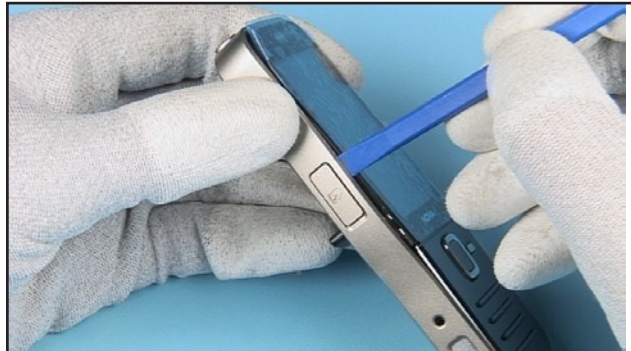
10. Gently pry open the clips of the WINDOW ASSEMBLY.
