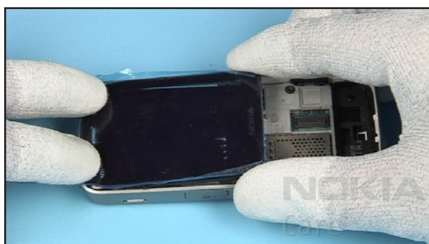
20. Click in the top snaps of the WINDOW ASSEMBLY.
