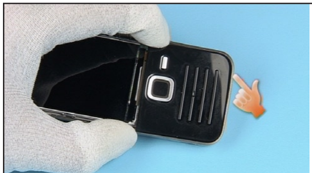
14. Push the UI MODULE ASSEMBLY sideways in order to reach a recess as shown.
