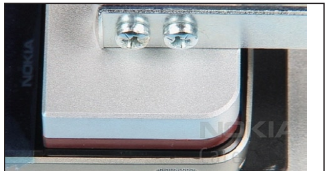
30. Wait at least 5 seconds to activate the adhesive before releasing the lever.
