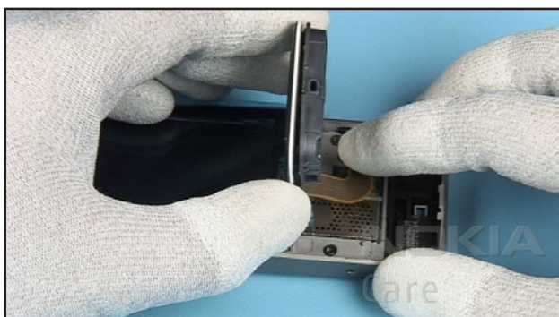
21. Close the flex connector of the UI MODULE ASSEMBLY.
