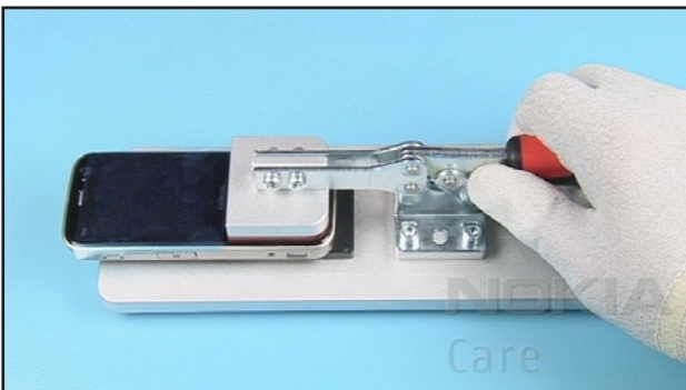
29. Slowly push down the lever completely.
