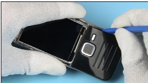
13. Gently pry open the clips at the shown side.
