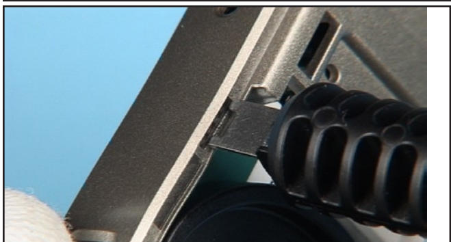
8. Insert the SS-149 Tool in order to unlock the clips of the UI MODULE ASSEMBLY...
