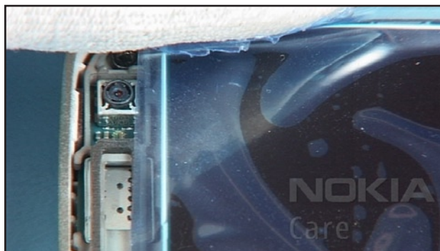
18. Position the LCD into its compartment.
