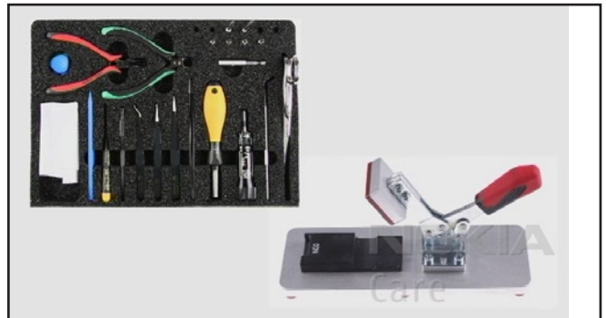
2. You will need the Nokia Standart Toolkit Version 2 and the SS-153 in case of replacing the SUPERKEY ASSEMBLY.
