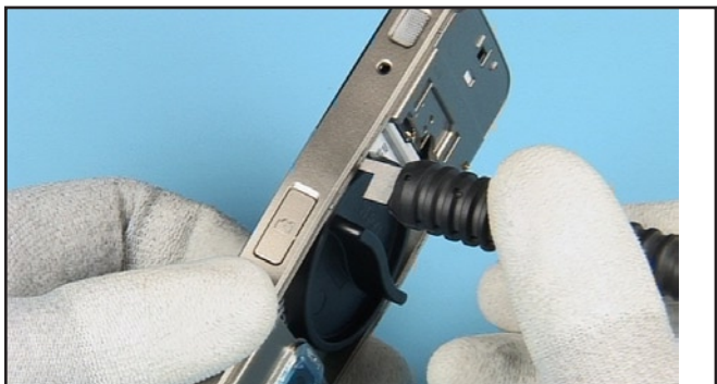
6. Start unlocking the clips of the WINDOW ASSEMBLY with the SS-159...
