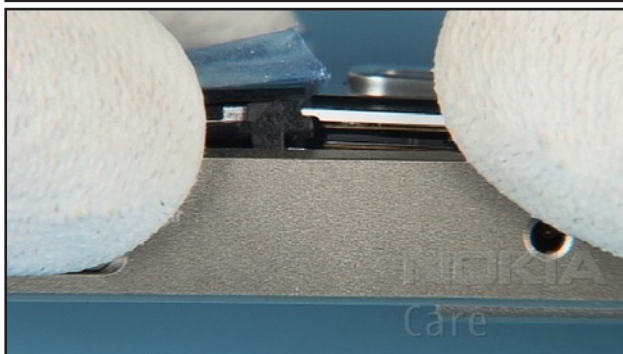
23. Align the UI MODULE ASSEMBLY with the WINDOW ASSEMBLY as shown.
