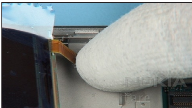
17. Bring the LCD near the Flex connector. Close the connector.
