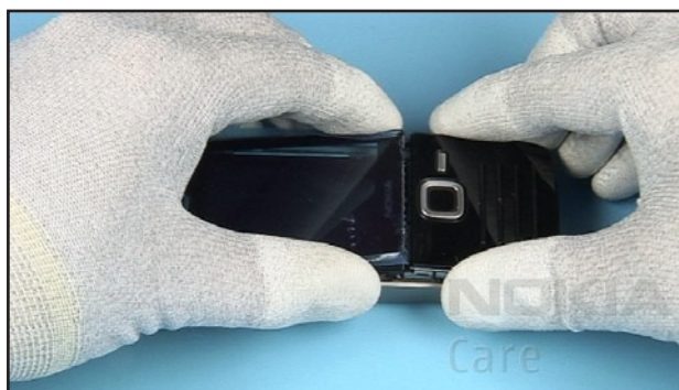
22. Gently push the rear clips of the UI MODULE ASSEMBLY into their places
