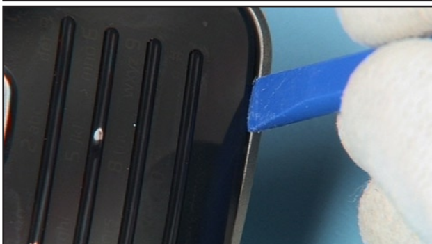
15. Insert the SS-93 into the recess and pry open the 2 clips.
