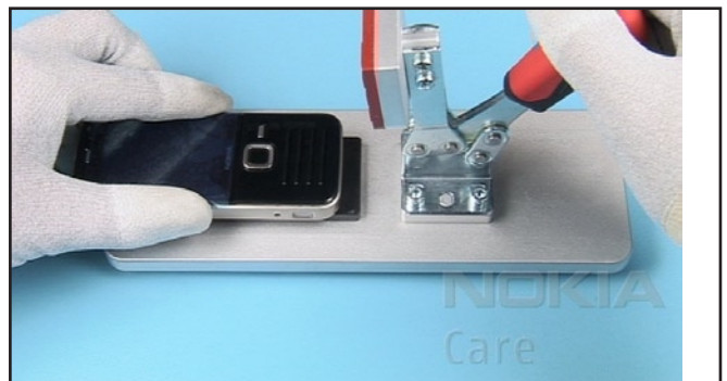
28. Insert the Assembly into the SS-153.
