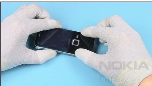
27. Remove the protective film. Align the SUPERKEY exactly to the UI MODULE ASSEMBLY.
