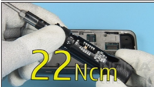
15. Set the correct torque.
