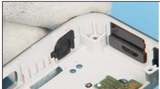
36. The keys can be pushed out easily.
