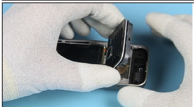
16. If the clips are released properly, the UI MODULE ASSEMBLY can be lifted up.
