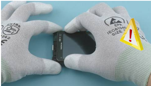
37) Carefully place down the WINDOW ASSY. Make sure that the connectors remain connected!
