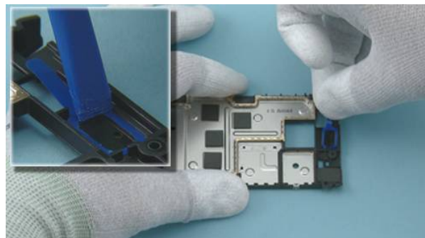
24) Place the EARPIECE ADHESIVE and activate the adhesive by carefully pressing down on it with the SS-93. Remove the blue EARPIECE ADHESIVE protective film.
