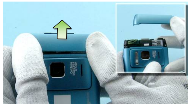
12) Remove the TOP COVER by pushing it from the back side to the direction shown.
