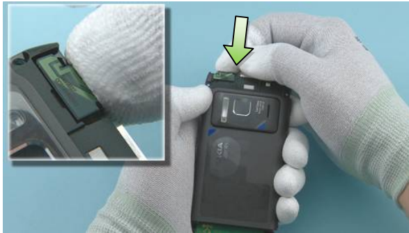
33) Push the COMBO ANTENNA into place.
