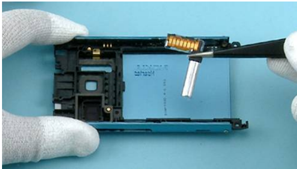
49) Remove the FLASH MODULE with the tweezers.
