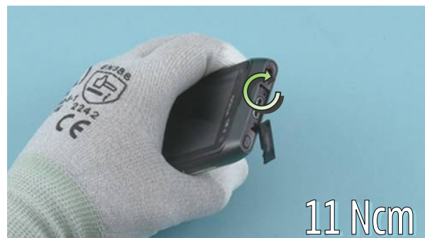
42) Tighten the TORX + size 5 screw to the torque of 11 Ncm.
