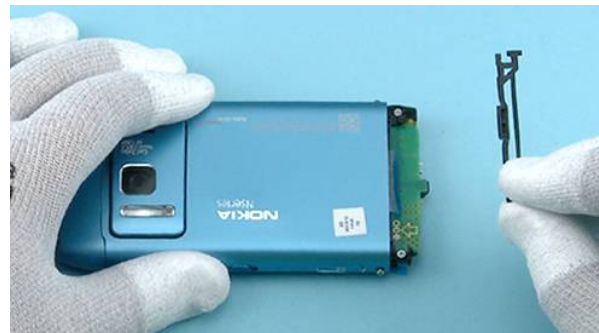
8) Now the BATTERY LID can be removed.
