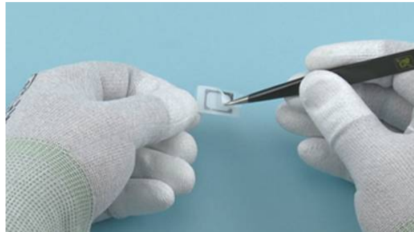
16) Remove the IHF GASKET protective film.
