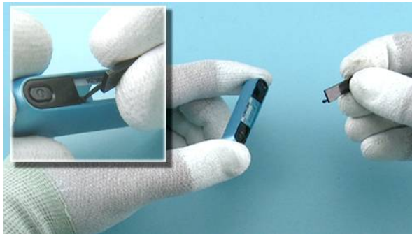
13) Pull out and remove the HDMI HATCH.
