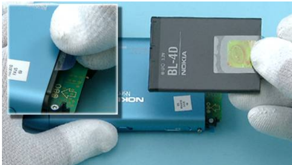
9) Pull out and remove the BATTERY by using the BATTERY PULL-OUT TAPE.
