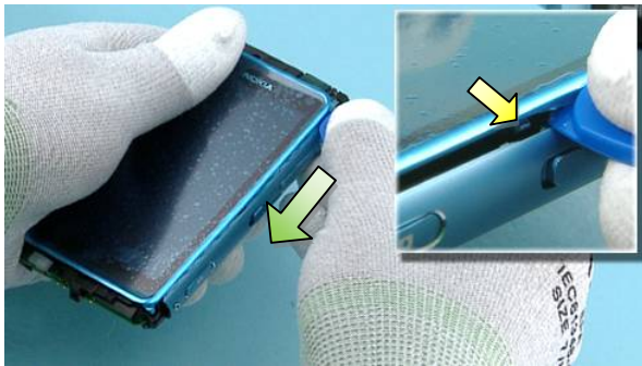
15) Slide SRT-6 to the direction shown to release the clip holding the WINDOW ASSY.
