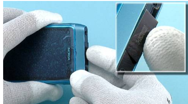
10) Open the HDMI HATCH.
