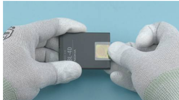
44) Place the BATTERY PULL-OUT TAPE to the BATTERY as shown. Press it down slightly to activate the adhesive.
