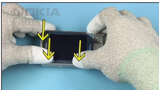
45. Close the snaps on the other side and the top side. Check that no gaps remain.
