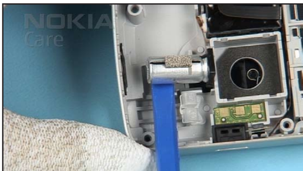
41. Carefully remove the CAPACITOR with the SS-93.
