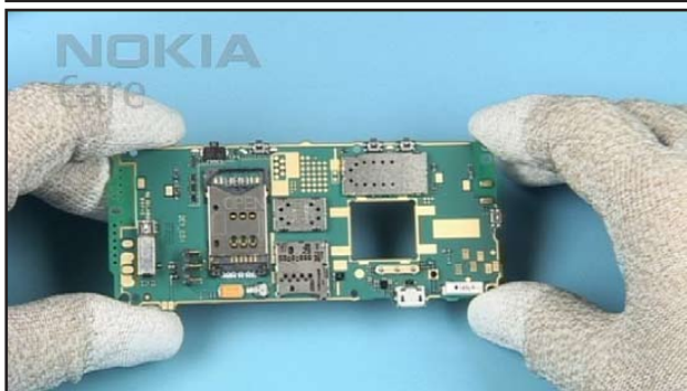
23. Check the mechanical condition of the spring contacts on the ENGINE MODULE.
