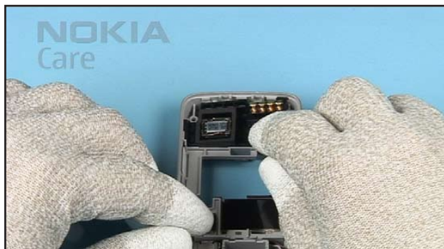
18. Press on the ANTENNA to secure it into place. Do not touch the spring contacts.
