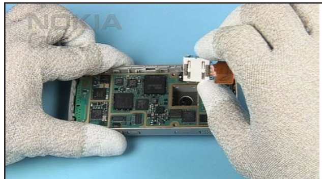
28. Fit the CAMERA MODULE.
