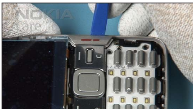
12. Unlock both side snaps. Avoid damaging of the B-COVER.
