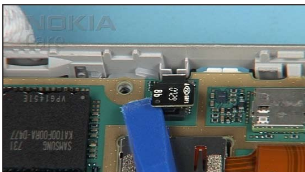
27. Carefully open the FLASH MODULE CONNECTOR.
