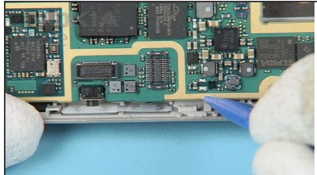
26. Press the ENGINE MODULE into place. Take special care to the electric components.
