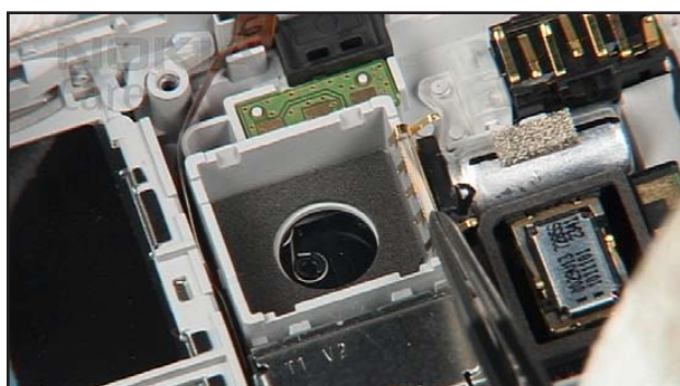
20. Carefully fit the CAMERA GROUNDING SPRINGS.
