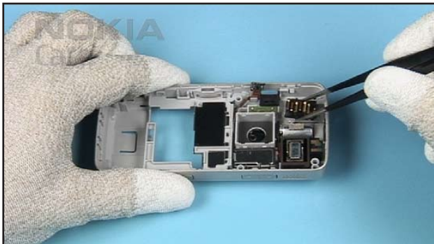
15. Place the AUDIO CONNECTOR into the B-COVER...
