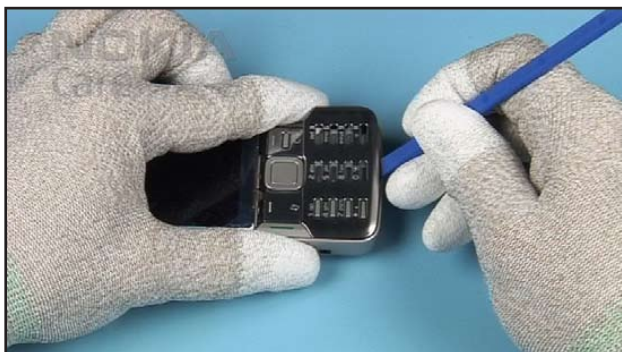
9. Unlock all clips of the KEYMAT COVER.
