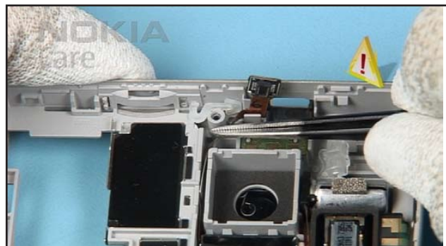
12. Check the correct position of the flex connector.
