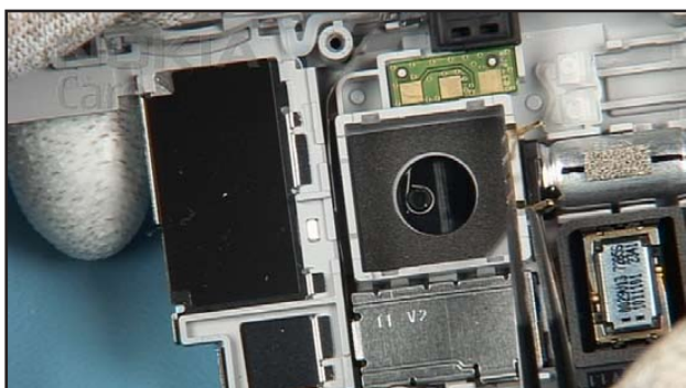
37. Carefully remove the CAMERA GROUNDING SPRINGS.
