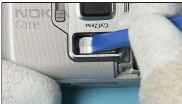
42. Remove the FLASH from B-COVER.
