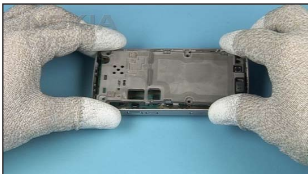
25. Remove the MAIN FRAME ASSY from the B-COVER.
