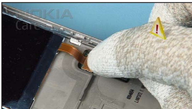
33. Close the LCD connector.
