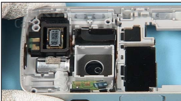
11. Fit the FLASH MODULE by carefully pressing it into B-COVER. Ensure that the flex foil is not bend or squeezed.
