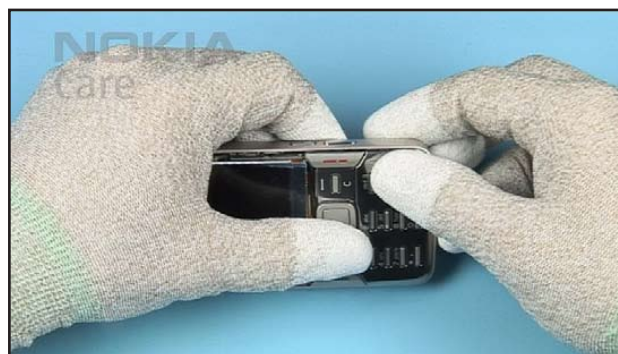
38. ...and press it into place. Check that no gaps remain.
