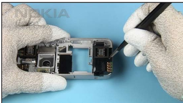
17. Place the ANTENNA CELLULAR ASSY into the B-COVER.
