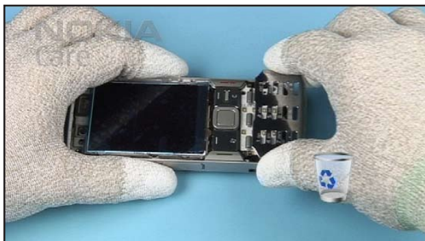
10. Remove the KEYMAT COVER and discard it.
