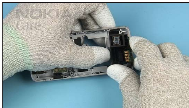
34. ...and remove it from the B-COVER.
