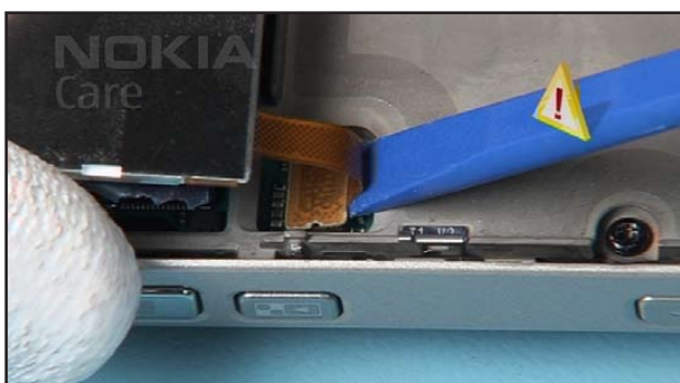
19. Gently open the LCD connector.
