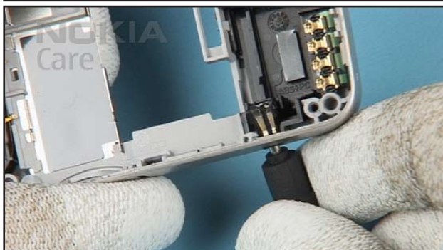
31. Remove the DC-JACK with the DC-Plug.
