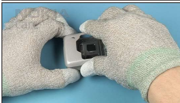
48. Move the D-COVER a bit to the left and remove it.
