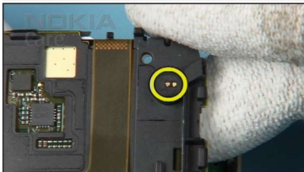
16. Remove the MICROPHONE and discard the UI MODULE.
