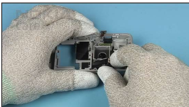
43. Carefully remove the FLASH MODULE...
