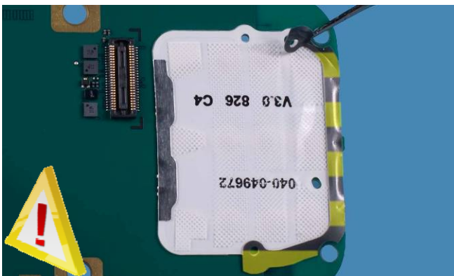
17) Use a dental pick to release the LIGHT BLOCK TAPE .
