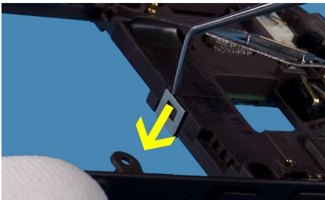
21) Use a dental pick to release the 2 nd PWB FASTENER .
