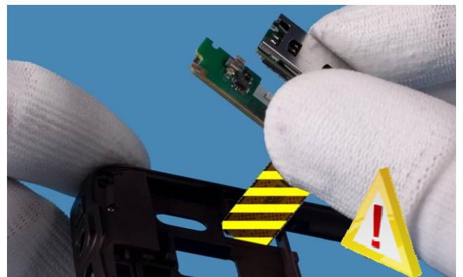
24) Remove the 2 nd PWB . Be careful with the CONNECTION FLEX .
