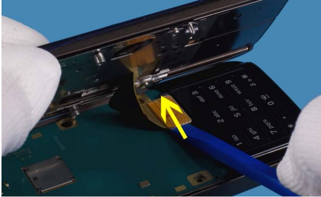
7) Lift up the upper block and use SS-93 tool to release the connector of the LCD.
