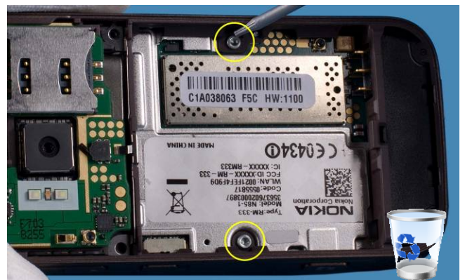
6) Unscrew the two screws with a TORX 4+ screwdriver.
