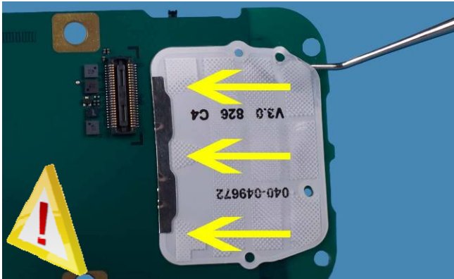
19) Release the DOMESHEET with a dental pick.
