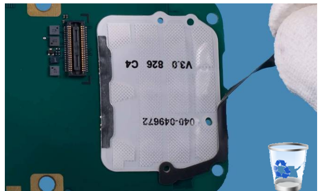
18) Peel off LIGHT BLOCK TAPE . Do not use it again.
