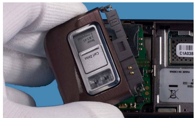
4) After releasing the screws remove the BACK COVER .
