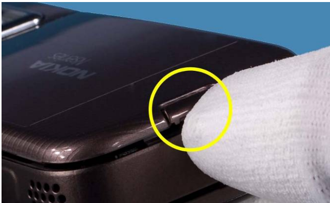
1) Push button and unlock the BATTERY COVER .
