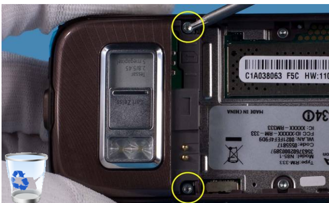
3) Unscrew the two screws using a TORX 6+ screwdriver.
