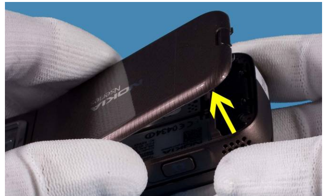
2) Lift up and remove the BATTERY COVER .
