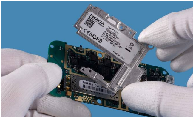
15) Separate the BB SHIELD from PWB .
