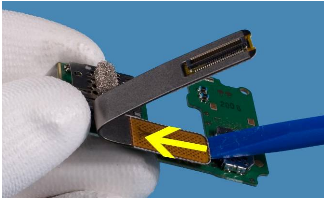
25) Open the connector of the CONNECTION FLEX and remove it.
