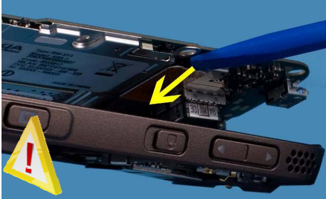
13) Carefully lift up the PWB and open the connector using SS-93 tool.
