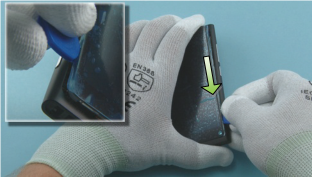
13) Use the SRT-6 to open the right side of the DISPLAY ASSEMBLY.
