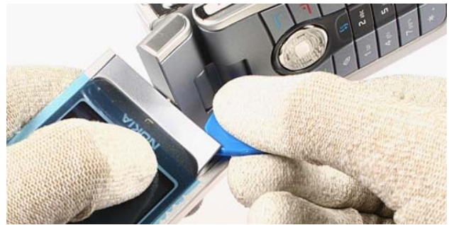
4.) The glued B-Cover Trim covers two screws. Release and remove it with the SRT-6.
