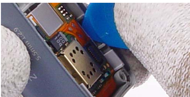
17.) Release the Audio Cavity with the SRT-6 carefully.
