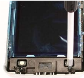
10.) Remove 2 Torx size 6 screws. For assembly use a torque of 19 Ncm.
