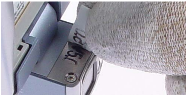
5.) Peel up the Cosmetic Layer on both sides.
