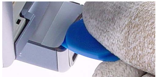
4.) The screws are hidden behind two glued Cosmetic Layers . Use new ones when reassemble.
