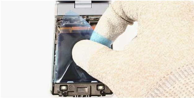
9.) Protect the LCD with a plastic film.
