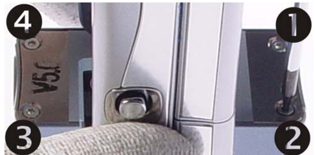
6.) Release the 4 Torx size 5 screws. The camera window is located on the left side in this picture. For assembly use the reverse order and a torque of 16 Ncm.
