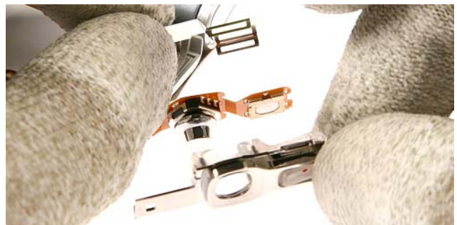
20.) Separate the Retainer plate from the Side Key Bezel Assy .
