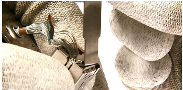
12.) Disconnect the connector with the SS-57 tool.
