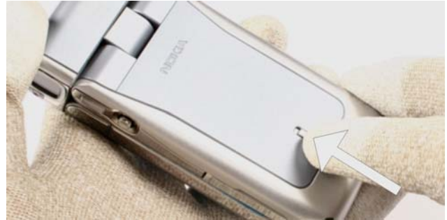
2.) Unlock and remove the Battery Cover . Ensure that no Battery is inserted.
