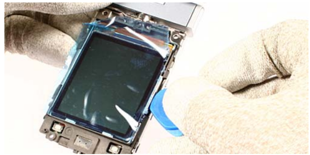
12.) Carefully release the Inner K2 LCD from adhesive.
