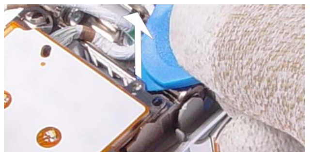
24.) Lever up the BB Shield Assy at the guidance as shown.
