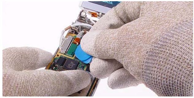
26.) Open the flex connector.
