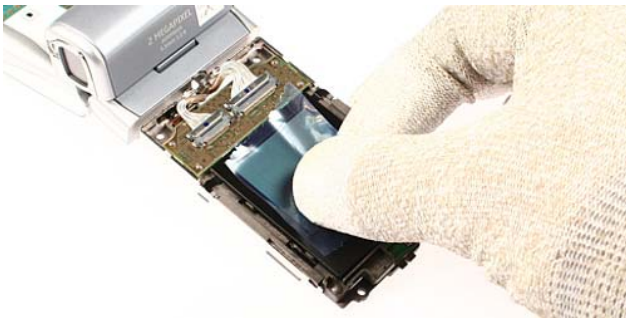
13.) Turn the unit and protect the Outer LCD with a plastic film.
