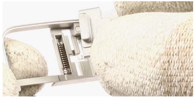
36.) Take away the Battery Cover Release Button . Mind the spring.
