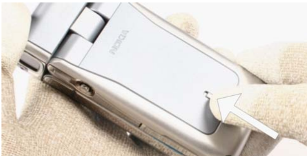
3.) Unlock and remove the Battery Cover . Always ensure that no battery is inserted.
