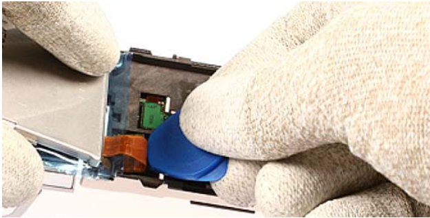
17.) Release the flex foil connector of the Inner K2 LCD .
