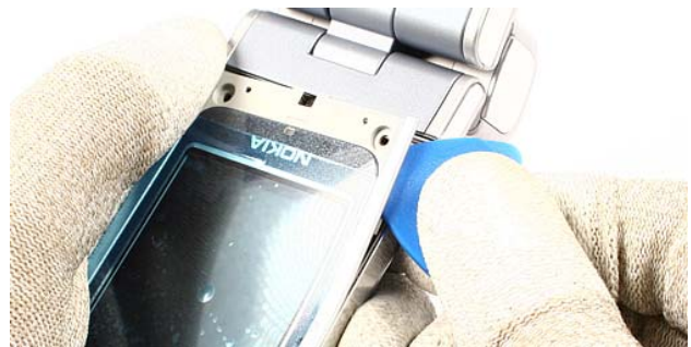
6.) Unlock all clips of the B-Cover with the SRT-6.
