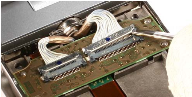
19.) Release the connectors from one side first.
