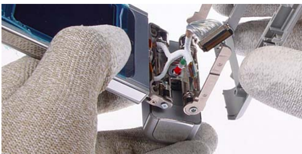
31.) Release the H-Cover from the Hinge.
