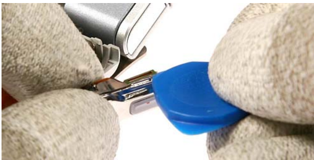
19.) Unlock the clips of the Retainer Plate .
