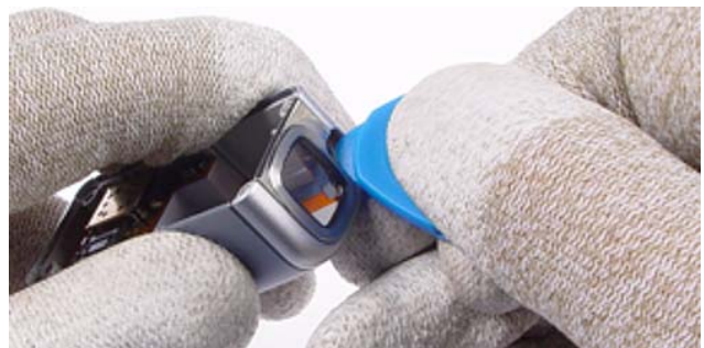
14.) Push the LED Window with the SRT-6 inside.
