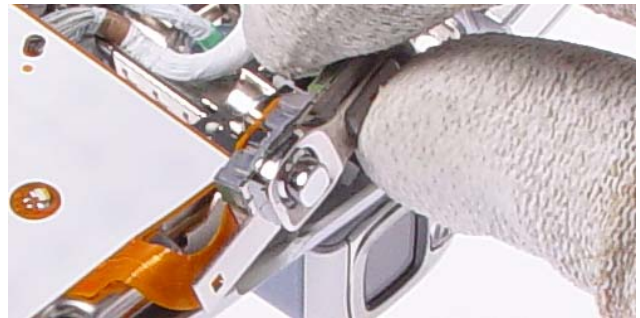
18.) Lift up the Side Key Assy . Mind the Flex foil.
