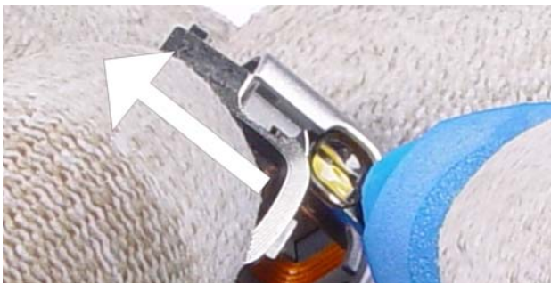
15.) And pull the Camera Bezel upwards.
