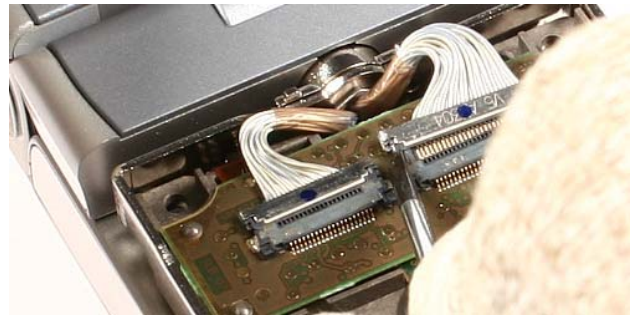
20.) Prevent scratching the PWB while releasing both connectors.
